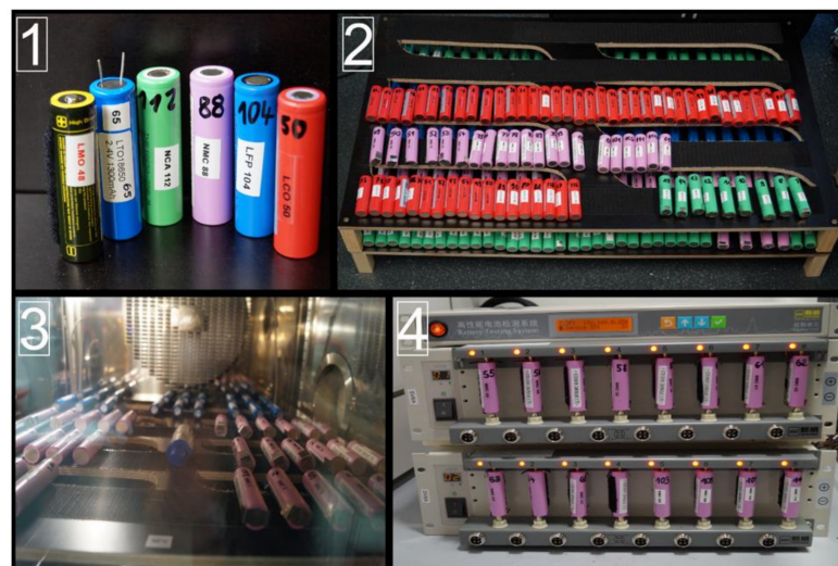
Figure 2. Panel 1: Selected cylindrical cells for the investigation; Panel 2: Wooden shelf construct for storage in climate chambers; Panel 3: Cells in climate chamber, including an additional temperature recorder (ELV USB-Datalogger UTDL10); Panel 4: Cells in four-wire clamps during capacity verification in tester.
