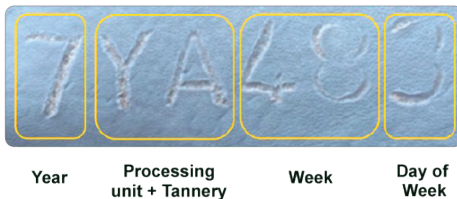
Fig. 3.5.1) Illustration of a "Leather ID" lasered into a hide (photo: JBS360; https://jbs360.com.br/en/leather-id/ )
