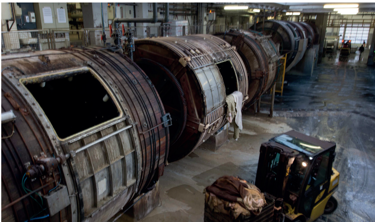
Fig. 3.2.2) Tanning drums (photo: Südleder & Ecopell)
