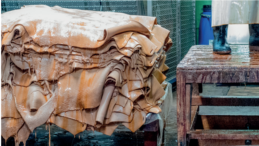
Fig. 3.2.4) Hides after vegetable tanning process (photo: Nina Conrad, btrr GmbH)
