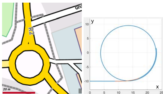
Figure 2: Curve radius comparison: Left – typical traffic roundabout. Right – Transition phase in comparison to complete turn
