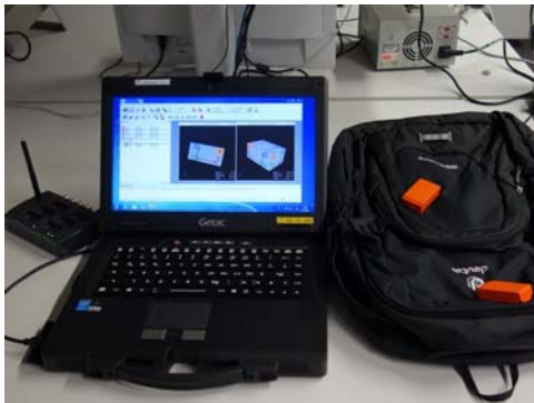
Figure 6: Wireless Data Acquisition and Evaluation with a ruggedized laptop computer
