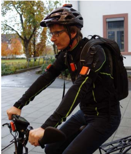
Figure 5: Multi axial inertial sensors (motion trackers) for analysing the dynamics of e bike and rider
