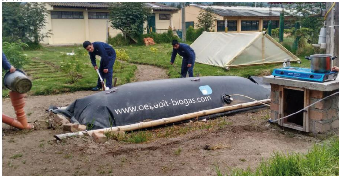
Figure 1. HoMethan system, fill-in unit (left side), two stirrers in the middle.
