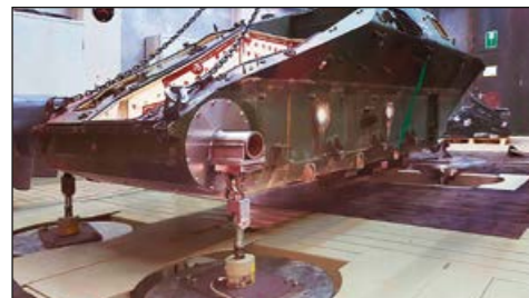
Fig. 1: Wiesel 2 hull torsion measurement on a 4-actuator running gear test bench (WTD 41-GF 220)
