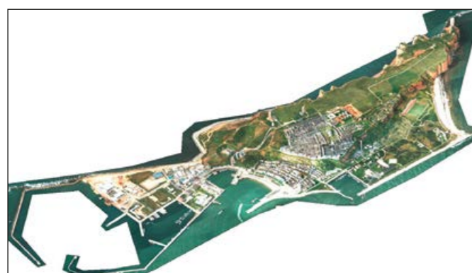
Fig. 1: Optical MACS dataset of the Island of Heligoland with a ground/spatial resolution of 5 cm, transformed to the radar image plane. The optical slanted view was calculated using the radar's imaging geometry as well as elevation data derived from the optical stereo dataset itself
