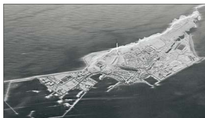
Fig. 2: Airborne F-SAR dataset for the Island of Heligoland with a ground/spatial resolution of 25 cm acquired in the X-band. The distinctive antenna mast at the image centre is absent in Fig. 1 because the wiry lattice structure of the mast did not lend itself to precise photogrammetric evaluation and induced an error in the elevation model
