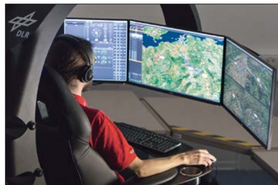
Fig. 1: HMI for the supervision and guidance of multiple UAS in controlled airspace
