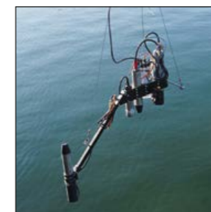
Fig. 5: DLR measuring system for spectral measurements (Source: DLR)
