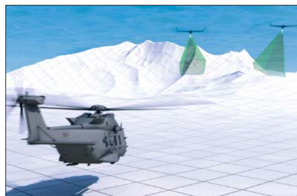
Fig. 1: Manned-unmanned teaming: Guiding multiple unmanned aircraft from the cockpit of a manned aircraft requires a high level of automation. An effective team comprising automation and humans is the key to successful missions
