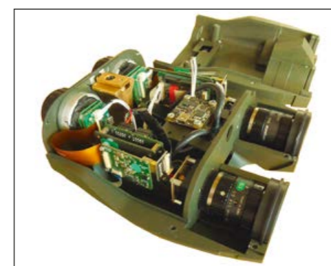
Fig. 4: Inside View of the VECTOR AR
