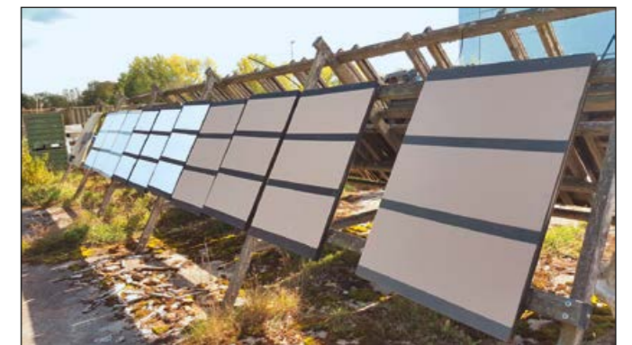
Fig. 4: Outdoor exposure test rig for weathering and stripping removable paints at the Bundeswehr Research Institute for Materials, Fuels and Lubricants
