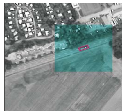
Fig. 3: LUNA video frame with visualisation of the automated object tracking process: box (magenta) around the tracked object, and image area analysed by the tracking technique (transparent cyan)
