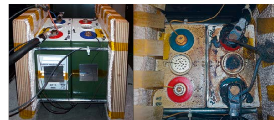
Fig. 4: Propagation test by means of overcharging, involving two charged LFP cells. Left: before the test, right: after the test. The passive cell failed to catch fire itself during the thermal runaway of the neighbouring overcharged cell
