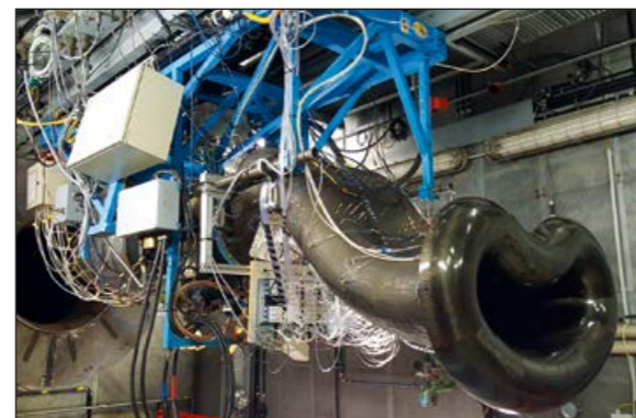
Fig. 2: Experimental set-up with installed MEIRD intake system and Larzac 04 engine in the engine test facility at the Institute of Jet Propulsion
