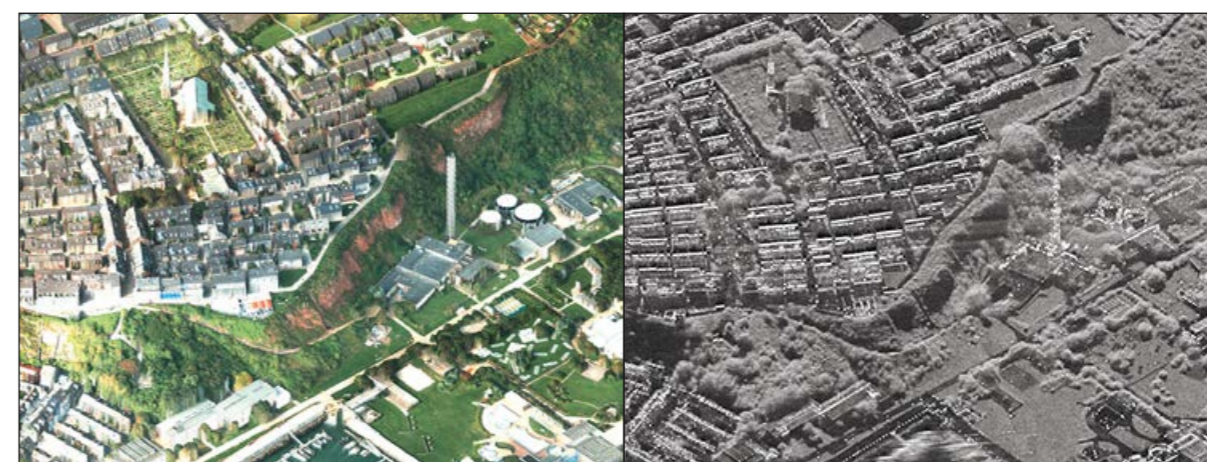
Fig. 3: Details in the central urban region of the island. The pixel-exact alignment of the respective datasets is clearly visible both for topographic features such as the rock cliffs and for urban structures like the church, village buildings and large lattice mast
