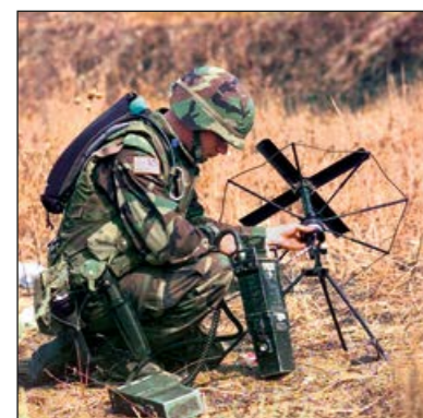
Fig. 1: Man-pack UHF satellite radio for links via geostationary satellites, as currently used in the Bundeswehr (Source: nara.getarchive.net)
