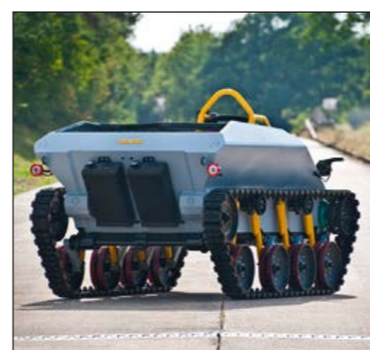
Fig. 3: WEASEL HYDROP: With a ground clearance of 400mm, it has 100mm greater spring travel than the Wiesel 1
