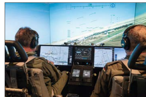
Fig. 3: Conducting an MUM-T experimental campaign in a helicopter mission simulator to evaluate the adaptive associate system
