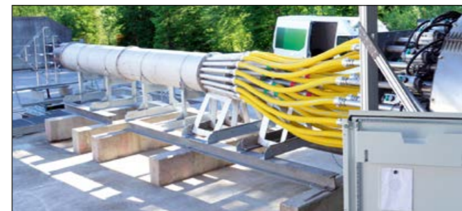
Fig. 2: Air flow pipe on the test rig (courtesy of WTD 52)
