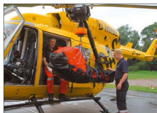
Fig. 3: Survival kit attached to a helicopter hoist cable
