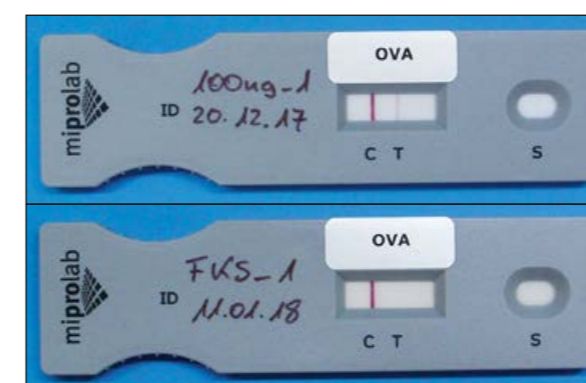
Fig. 3: LFA: Testing of sensitivity with ovalbumin solution (100 ng/ml), and testing of specificity (cross-reactivity) with fetal calf serum (FCS)
