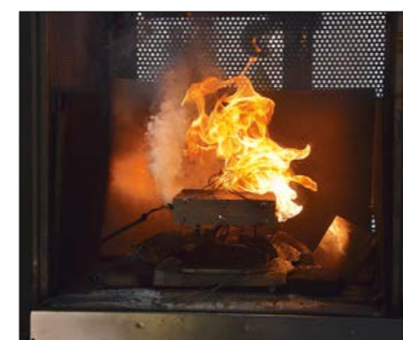
Fig. 3: Electrolyte release and fire during thermal abuse testing of a lithium ion cell
