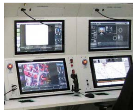
Fig. 1: ABUL video exploitation system in the LUNA UAS ground control station, on the dual monitor to the left
