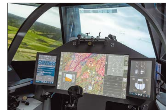
Fig. 4: With the aid of eye tracking and other sensors, the crew's activities are recorded contact-free and non-intrusively and combined with model knowledge to provide task-specific support
