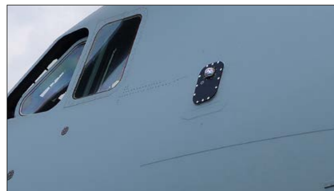
Fig. 1: Exterior view of a MIRAS warning sensor installed in an Airbus A400M of 62 Air Transport Wing
