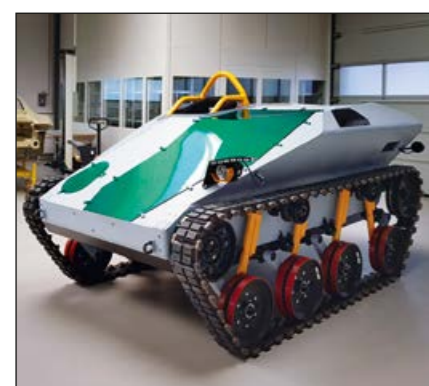
Fig. 1: WEASEL HYDROP: The track rollers and return rollers are made of CFRP (Capricorn Composite GmbH)
