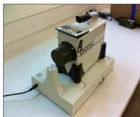
Fig. 1: Micro-Detective, a mobile radiation-detection system for rapid radionuclide identification based on gamma spectroscopy (Ortec, Oak Ridge, USA)
