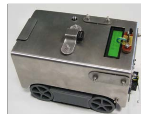
Fig. 3: Autonomous model. Vehicle with infrared navigation and LCD display for status indication, light detection, and sensor for measuring the radioactivity
