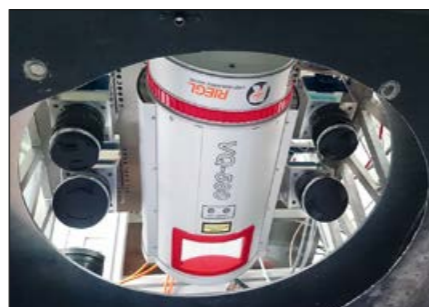
Fig. 2: Airborne laser scanner RIEGL VQ-580 (Source: Fraunhofer IOSB)
