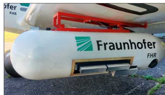
Fig. 1: MIRANDA-35 radar sensor mounted under the wing of an ultralight DELPHIN aircraft
