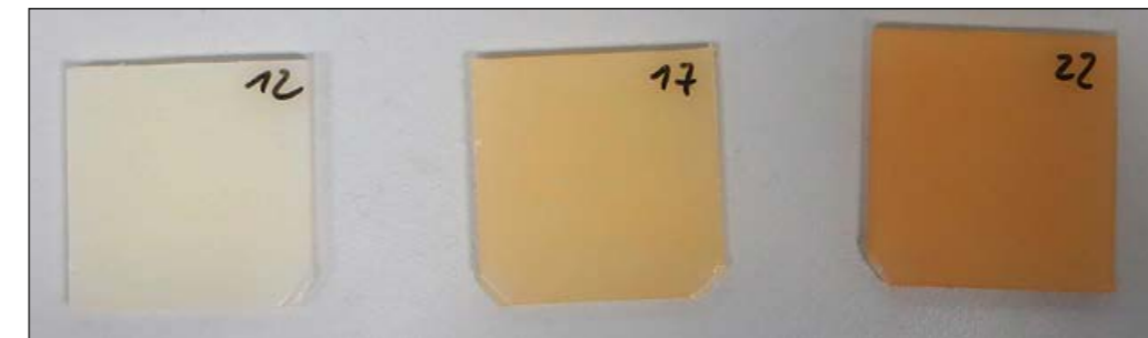
Fig. 3: Artificially aged polymer samples. A strong change in colour is evident
