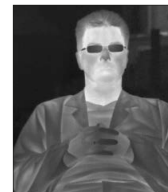
Fig. 4: Thermal image delivered by a 640 \times 512 LWIR superlattice camera operated in this instance at a high temperature of 90 K. To date, the only European manufacturers in a position to demonstrate such a performance capability are cooperation partners Fraunhofer IAF and AIM Infrarot-Module GmbH
