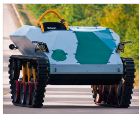
Fig. 2: WEASEL HYDROP: Bonnets and covers are made of aluminium foam sandwich AFS (pohltec metalfoam GmbH)
