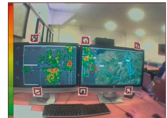
Fig. 4: Aggregated fixations (heatmap) during an engine failure situation in the first simulation study
