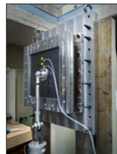
Fig. 2: Life testing on a servo-hydraulic vibration test bench (WTD 41-GF220)
