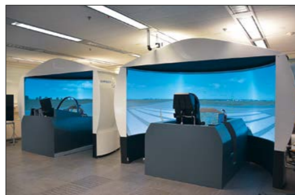
Fig. 2: The FCAS/NGWS MUM-T simulator of the Institute of Flight Systems is used for testing novel assistance, planning and mission functions. Two single-seater or, alternatively, one twin-seater cockpit can be used to simulate different cockpit configurations
