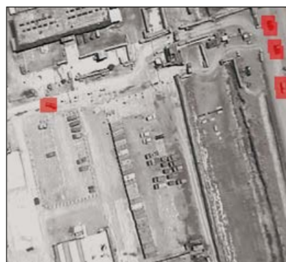
Fig. 2: LUNA video frame with overlay highlighting the automatically detected moving objects
