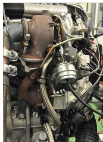
Fig. 1: WEASEL S38 engine with two-stage Borg Warner Turbo Systems R2S charging assembly on the engine test bench (Trier University of Applied Sciences)
