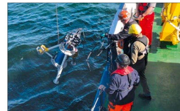
Fig. 3: Deployment of the blue bottom node by RV EMB
