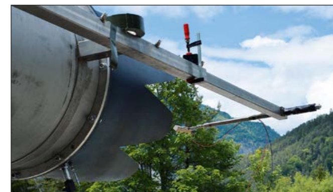
Fig. 3: Flare decoy ammunition on a fixed mount (courtesy of WTD 52)
