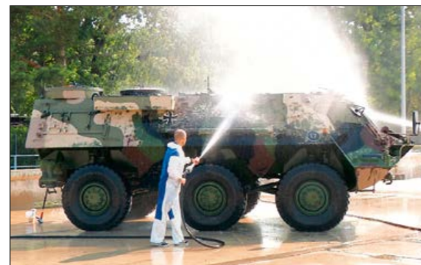
Fig. 2: Field-testing the stripping of removable paint from a Fuchs armoured carrier (APC)
