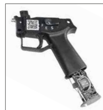
Fig. 2: First functional illustrator of a handgrip sensor system for recording the spatial orientation of a handgun using the modular G36 handle as an example
