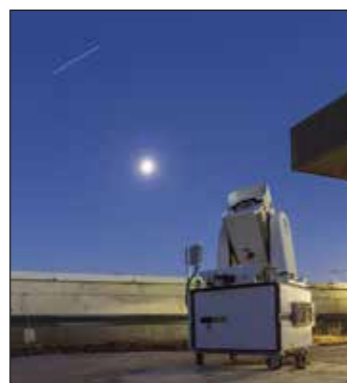
Fig. 2: Wide-angle camera system in weatherproof housing during field tests. Orbital objects like the International Space Station are detected as short streaks
