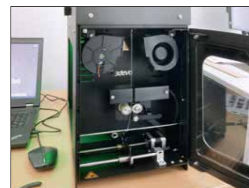
Fig. 3: Final process step of filament production extrusion of recycled material and subsequent spooling
