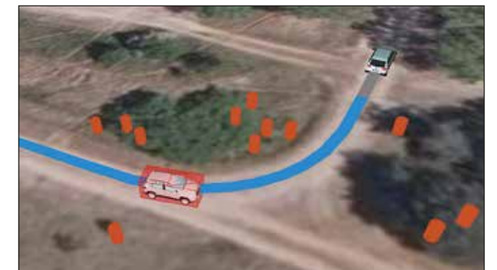
Fig. 4: The lead vehicle continuously transmits landmarks (red cylinders) and its path (blue line)
