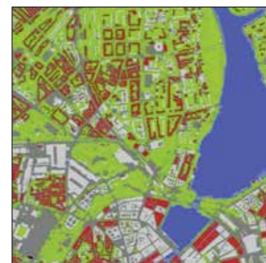
Fig. 2: Retrieval of material information from a satellite image. Color-coded material map for Fig. 1 (C); red: roof tiles, blue: water, light green: grass, dark green: trees, light grey: concrete, dark grey: streets
