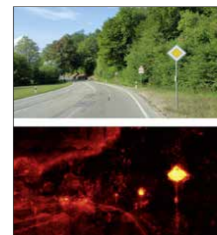
Fig. 4: A road section with traffic signs (top) and associated conspicuity map (bottom)
