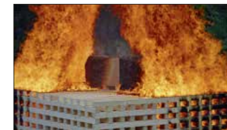
Fig. 5: Protective foam formation during bonfire test
