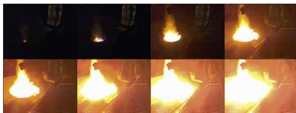
Fig. 1: Development of an artificial deflagration over time. The time between the images is 10 ms
