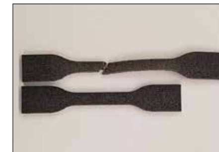
Fig. 5: Thermoplastic polyurethane estane 3D TPU M95-A from multijet fusion after tensile test (top) exhibiting medium recovery to initial shape (bottom) (source: Vivianne Marie Bruère de Carvalho Paiva)
