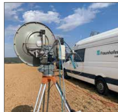
Fig. 3: Ground control station with telemetry antenna south of Bad Breisig during the 2020 measurement campaign with the Delphin ultralight aircraft
