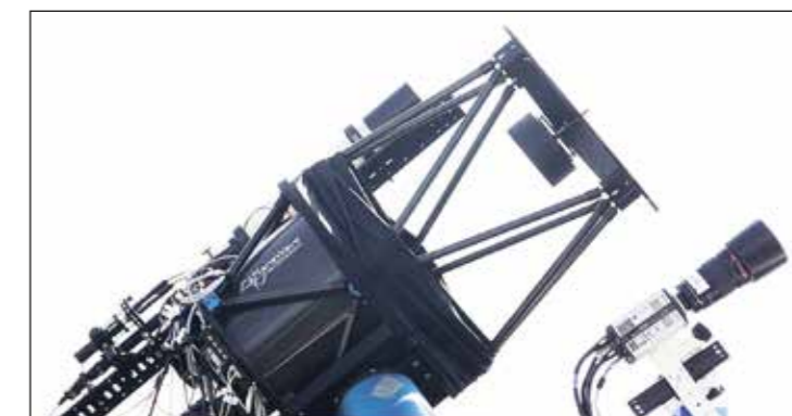
Fig. 5: Staring camera and 17-inch tracking telescope with mounted fibre-coupled laser transmitter
