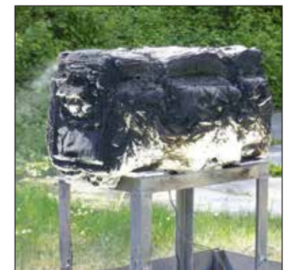
Fig. 6: Metal ammunition box after bonfire test
