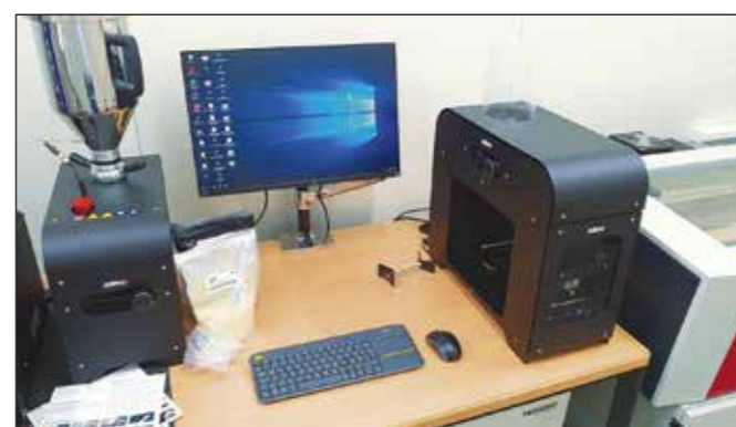
Fig. 2: Desktop filament production line with dryer (left) and extruder with integrated spooling system (right)
