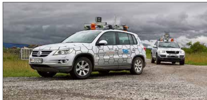
Fig. 1: MuCAR-3 and MuCAR-4 research vehicles from the Institute for Autonomous Systems Technology with roof-mounted lidar sensors
