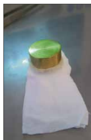
Fig. 3: Bonding of the nanofiber material to a metal cylinder representing the implant (source: Fraunhofer ISC)
