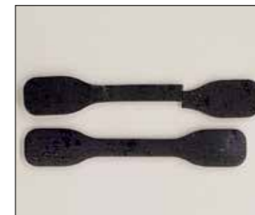
Fig. 4: Photopolymer TangoBlackPlus 70A from PolyJet after the tensile test (top) exhibiting high recovery to initial mould (bottom) (source: Vivianne Marie Bruère de Carvalho Paiva)
