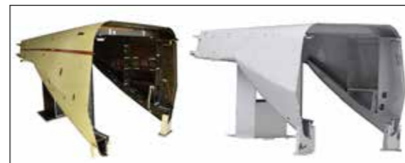
Fig. 3: Real NH90 tail structure on the left, CAD model created via 3D-scan on the right
