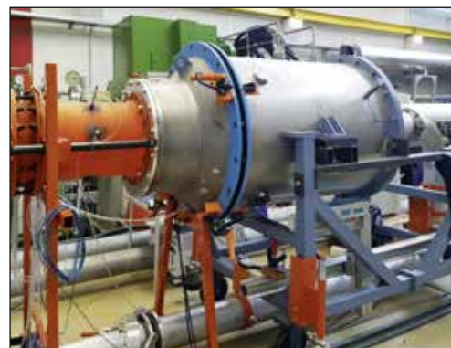
Fig. 1: Pressure vessel of the multi-purpose wind tunnel, mounted on a sliding carriage
