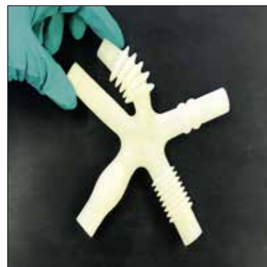
Fig. 1: High-strength silicone rubber component, 3D printing with material jetting (source: WIWeB)
