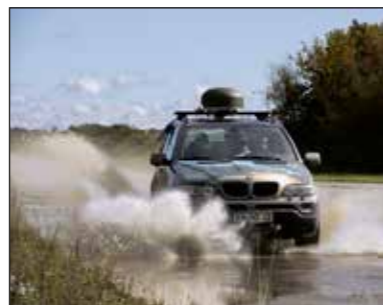
Fig. 2: SOTM terminal with phased-array antenna technology from ADS (source: ND SatCom, 2020)
