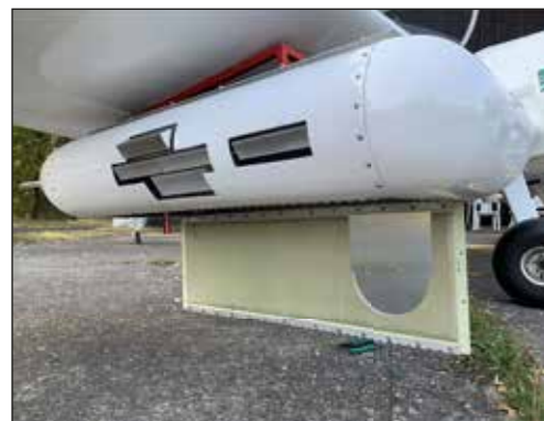
Fig. 1: MIRANDA35-4Rx system in the wingpod of the Delphin ultralight aircraft. The four receiver antennas (left) and the transmitting antenna (right) of the radar front end can be seen
