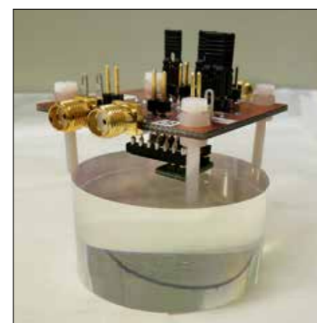
Fig. 3: Test of silicon photomultiplier electronics with an NE102A scintillator
