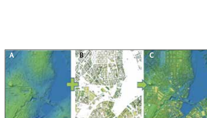
Fig. 1: Creation of a surface model for part of Hamburg (C) from a digital elevation model (A), building data (B) and a tree registry (not shown)
