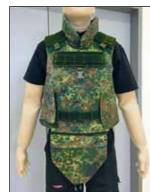
Fig. 3: Biofidelic dummy with a donned ballistic vest including special protection for the abdomen and neck
