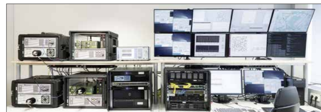
Fig. 3: Testbed for the real-time evaluation of radios consisting of the tested devices, the Multi-Layer Simulator with connection matrices, and position data generation (from left to right – source: Fraunhofer IIS/Paul Pulkert)
