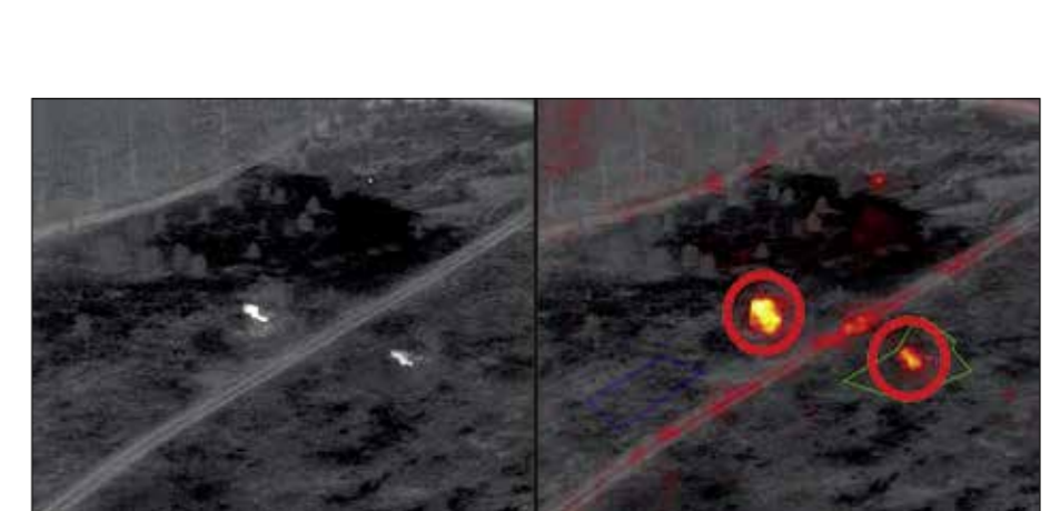
Fig. 5: Thermal image of camouflaged objects and the corresponding conspicuity map, which reveals differences, effectiveness and flaws in the camouflage
