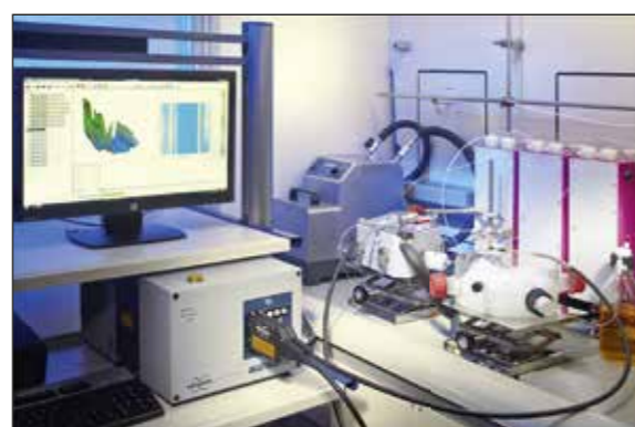
Fig. 2: Laboratory set-up for reaction screenings in microreactors with embedded spectroscopic process analysis using fibre optics
