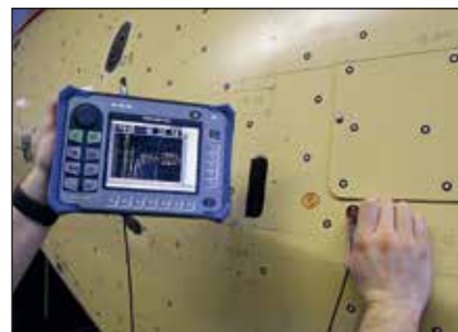
Fig. 1: Traditional state-of-the-art ultrasound inspection of a CFK structure
