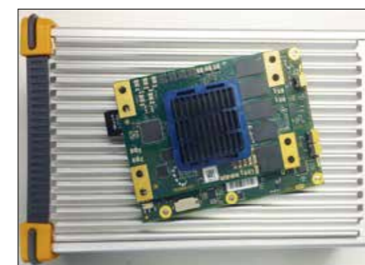
Fig. 2: Prototype HOD4Track demonstrator using Galileo PRS as a countermeasure to GNSS spoofing
