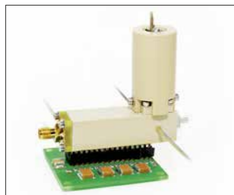
Fig. 1: Miniature IMS tube with non-radioactive ionisation source
