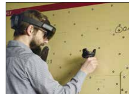
Fig. 4: AR-aided ultrasound inspection
