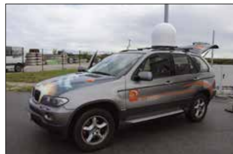
Fig. 1: SOTM terminal with traditional reflector antenna and with monopulse tracking approach from EM Solutions (source: ND SatCom, 2020)
