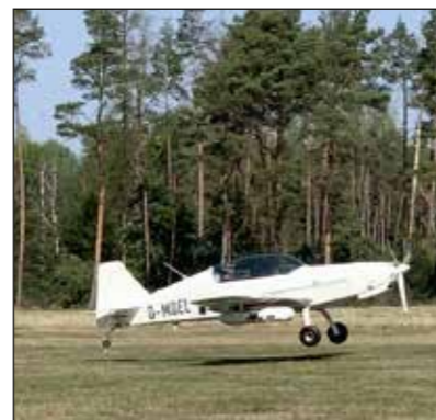
Fig. 2: Take-off of the Delphin ultralight aircraft at Mönchsheide airfield with MIRANDA35-4Rx integrated in the new wingpod
