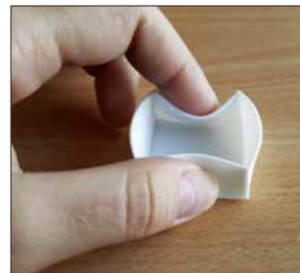
Fig. 3: Flexibility of a cube printed with thermo-plastic polyurethane 82A by FFF (source: Vivianne Marie Bruère de Carvalho Paiva)
