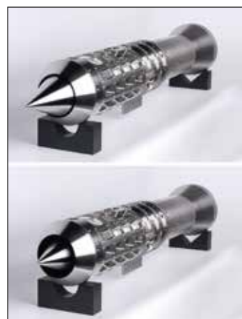
Fig. 1: Adaptive axisymmetrical air inlet model with extended (top) and retracted (bottom) central body
