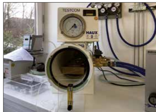
Fig. 2: Experimental hyperbaric chamber at the Naval Institute of Maritime Medicine
