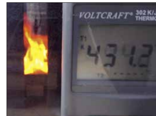
Fig. 3: Fast cook-off (fuel fire test)
