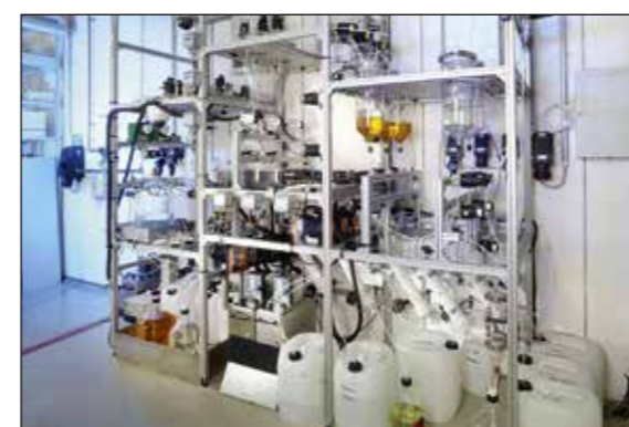
Fig. 3: Microreactor-based plant for the continuous synthesis and downstream processing of liquid explosives at a kilogram scale
