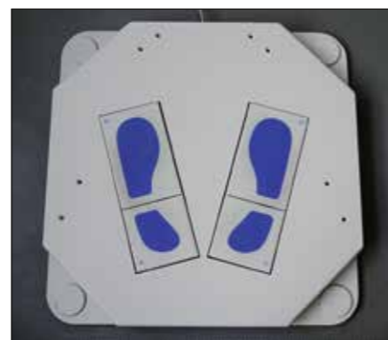
Fig. 3: Portable TETRIX Interactive Balance System made by Neurodata for measuring balance regulation (source: Dr. Carla Ledderhos, Bundeswehr)
