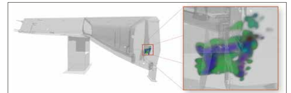
Fig. 5: Actual view of an auditor in a virtual environment. Ultrasound C-scan integrated in a semi-transparent CAD model
