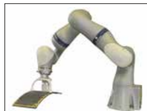
Fig. 2: Collaborative robot executing an ultrasound inspection of a CFK structure
