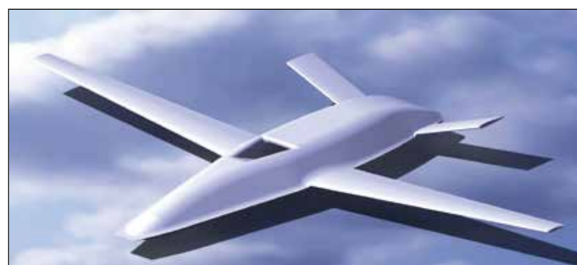
Abb. 2: Render einer Studie eines Unmanned Propulsion and Energy Research Aircraft
