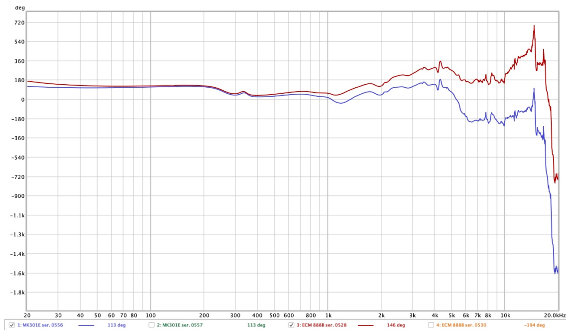
Fig. C.11: Phase frequency responses of both MKE301E (ser. 0556) and ECM888B (ser. E888B5A0528)
