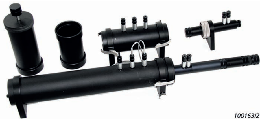
Fig. 3.2: The Brüel & Kjær Type 4206 Impedance Tube (Brüel Kjaer 2019: 1)
