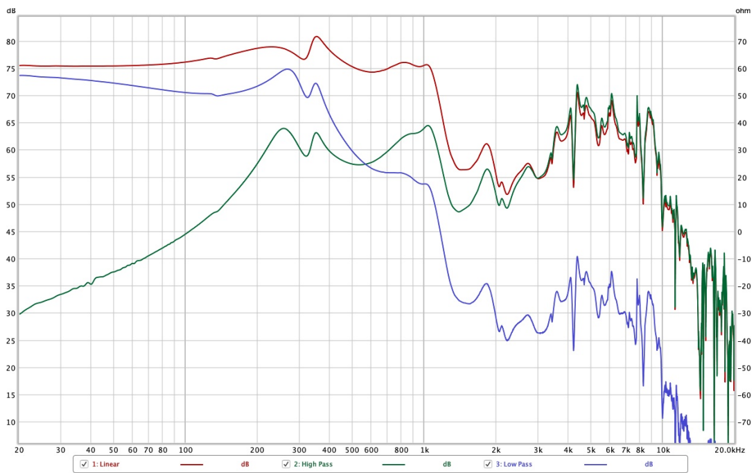
Fig. A.1: Comparison of amplitude frequency response of the three filter settings on the B&K 4206 impedance tube
