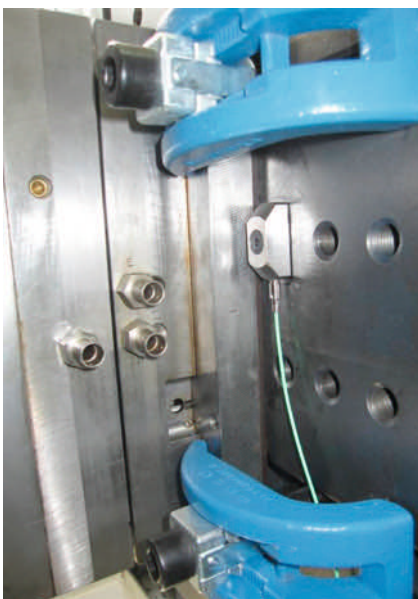
Fig. 4. The transducer is simply fastened to the fixed platen (figures: FHWS)
