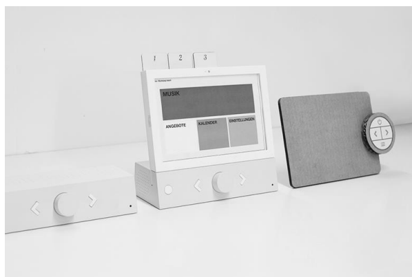
Figure 3: Three mock-up models for a workshop discussion with a haptic control unit
