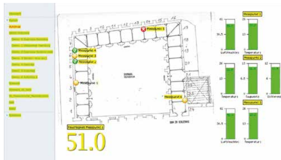
Figure 6: Visualization of the measuring points on site, defective devices are displayed in real time (measuring point 5).
