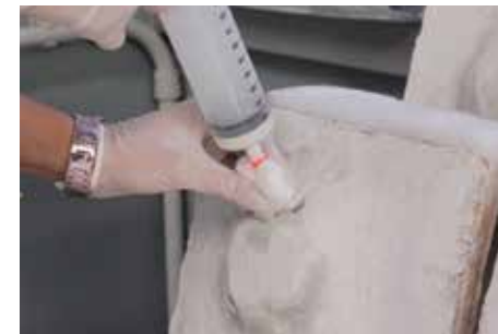
Figure 1: Injection of grout PLM25-75 into the replica of delaminated plaster
