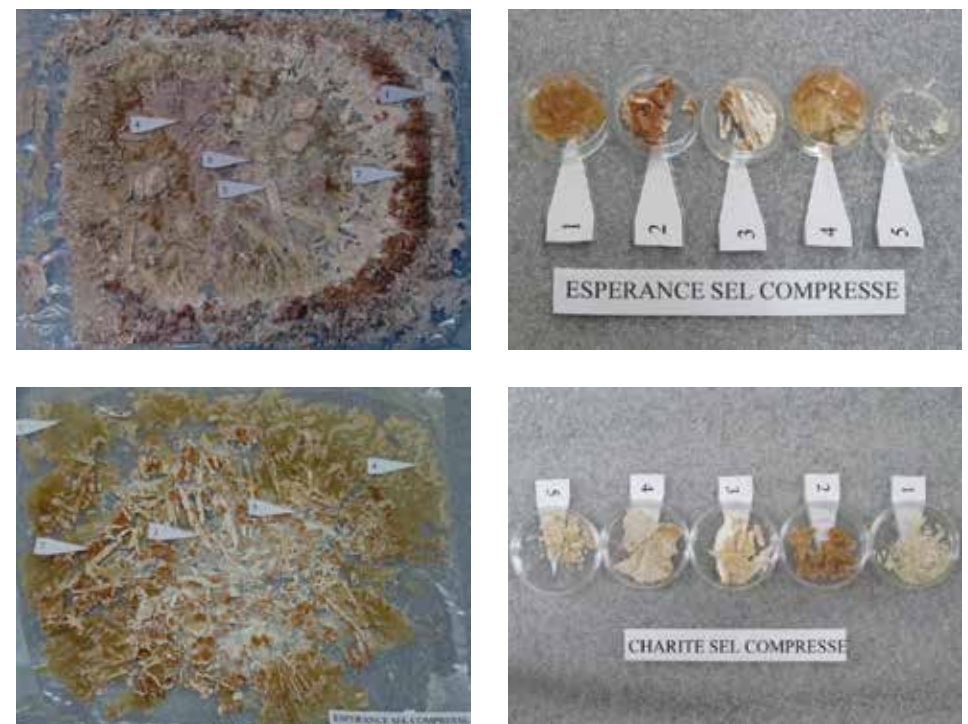
Figure 6: General aspect of the evaporates, and overview of the sampling.
