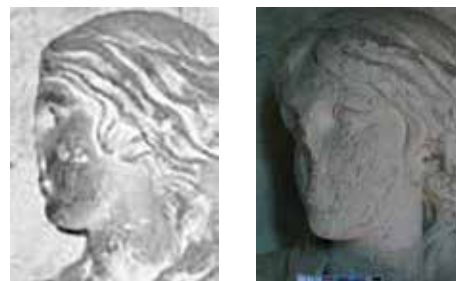
Figure 2: Face of the statue Esperance: blackening in 1998 (detail of figure 1), scaling and granular disintegration in 2012.
