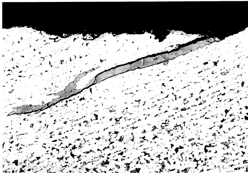
Fig. 2. Micro slice transverse to the defect [1].
