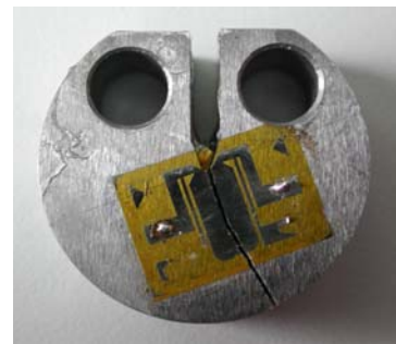
Figure 4. Specimen with 30° deviation between the direction of cold working and of the notch
