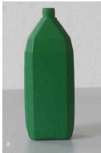
Figure 2. Visible (a) and SW IR (b) images (InGaAs camera) of a plastic bottle partly filled with room temperature water. The bottle is opaque in the VIS spectral range but partly transmits SW IR radiation.
