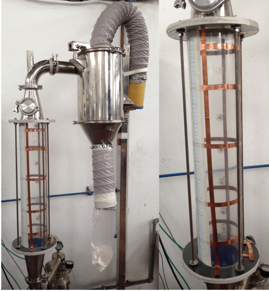
Figure 4.12: Experimental setup for the fluidization of the biomass samples.
