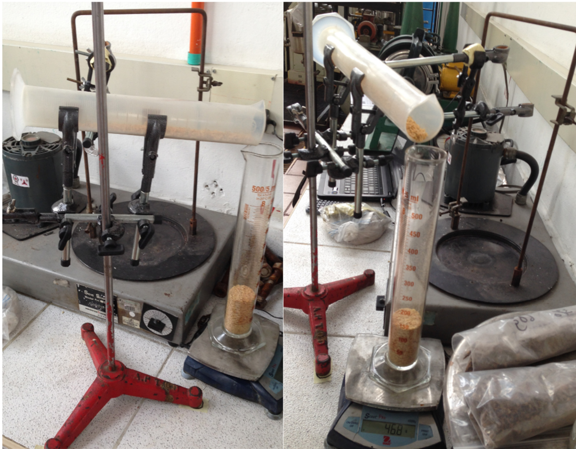
Figure 4.7: Experimental setup used for bulk density determination.
