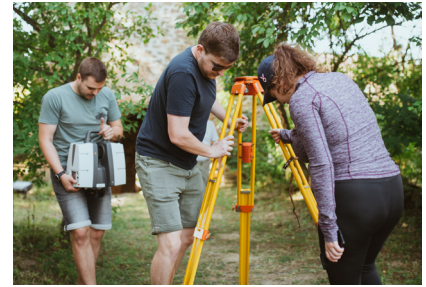
Fig. 3: Installation of the P40 terrestrial laser scanner from Leica.
