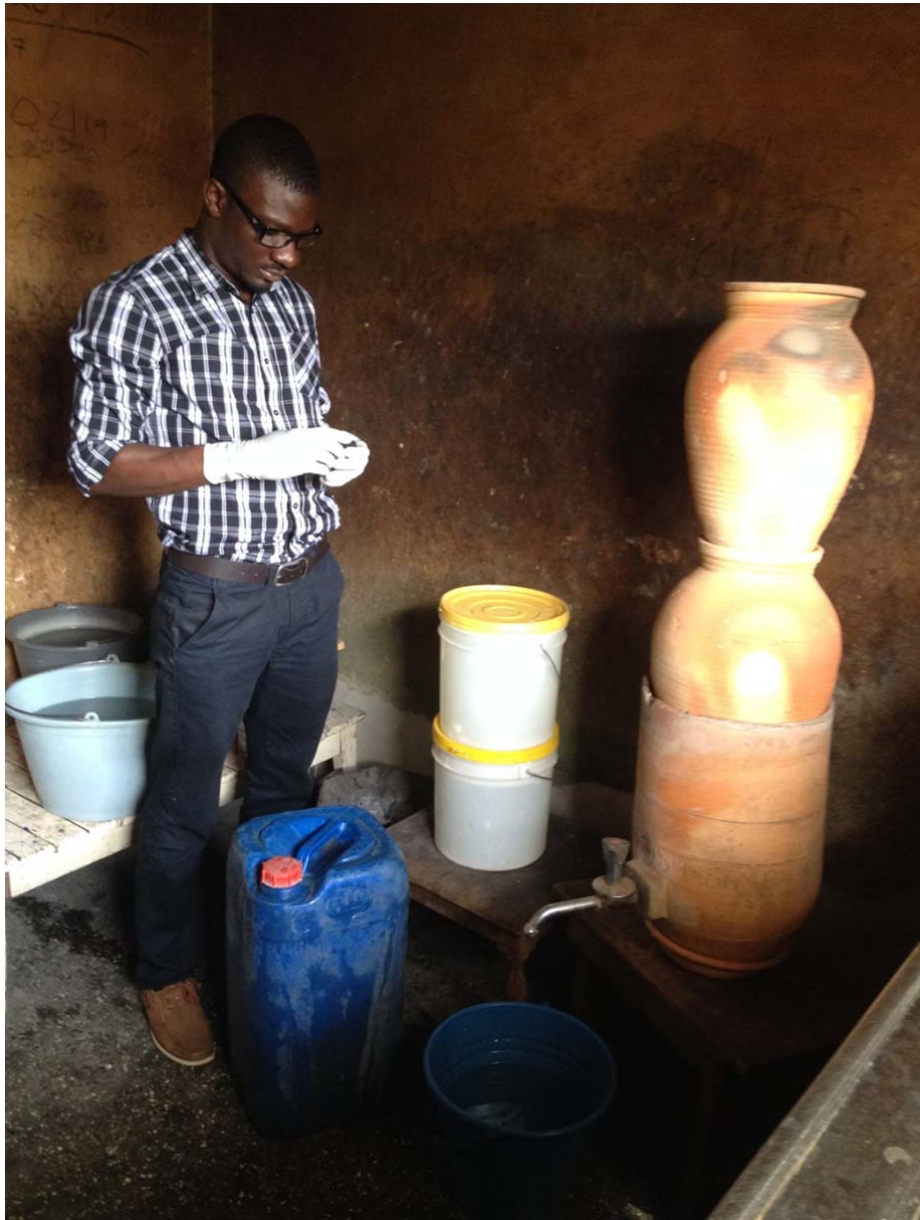
Figure 5.2: The actual three-earthen pot arsenic removal system used in this study.
