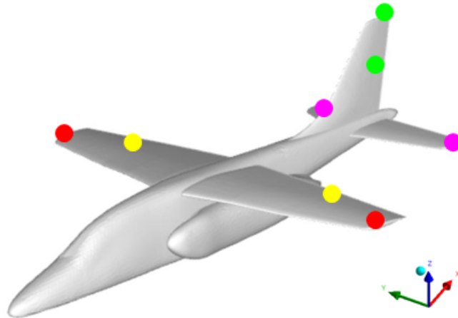
Figure 3.24: Mass configurations of the method demonstrator; colors denote variants according to Table 3.10: 1) red, 2) red + yellow, 3) green, 4) violet, 5) green + violet [65].
