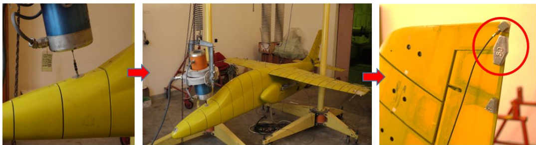
Figure 3.15: Iryda I22 experimental flutter model during GVT tests at the Institute of Aviation in Warsaw.
