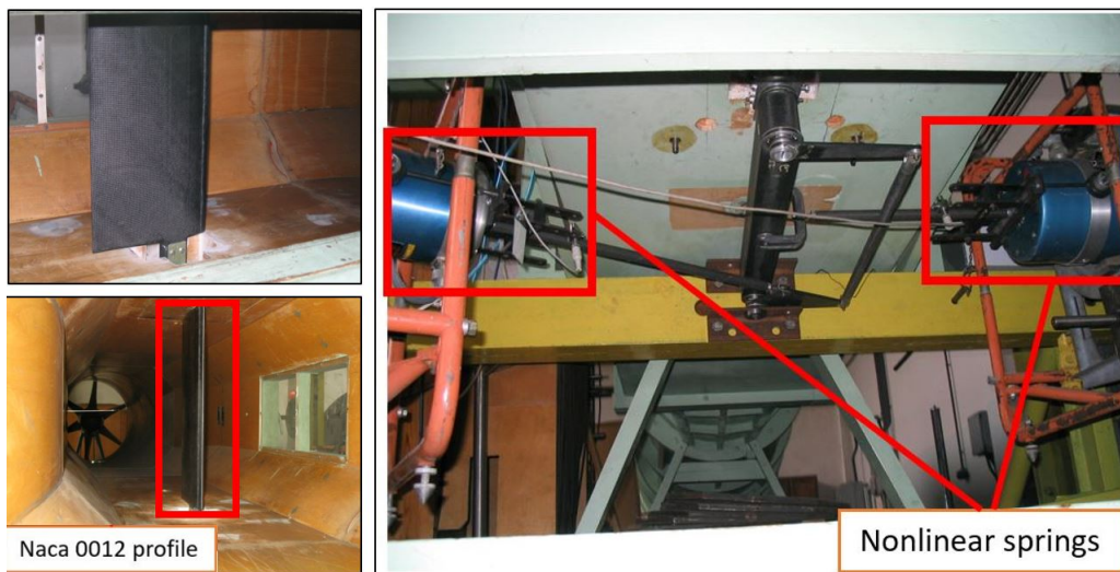
Figure 5.4: View of the testing setup in the wind tunnel of the Naca0012 profile
