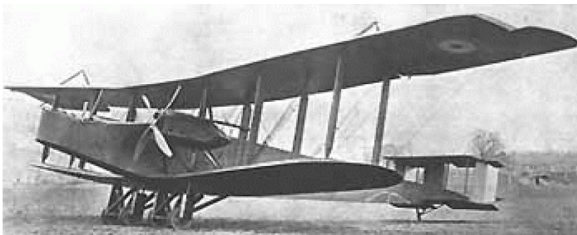
Figure 1.4: The problem of aeroelastic phenomena for the plane (1916) - caused by the lack of stiffening of outer section of the wing [58].
