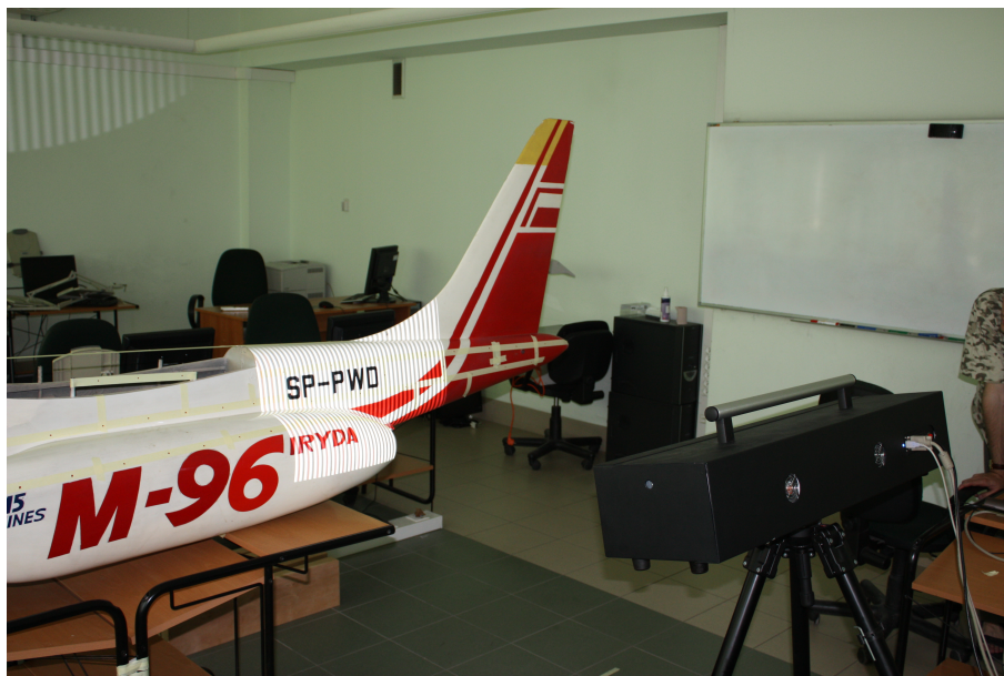
Figure 3.3: Optical scanner ScanBright during the measurement of the method demonstrator – Laboratory of Virtual Engineering [78]
