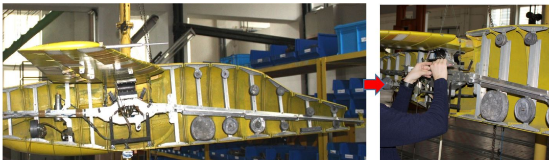
Figure 3.2: Measurements of the flutter model to correct the missing data in the documentation
