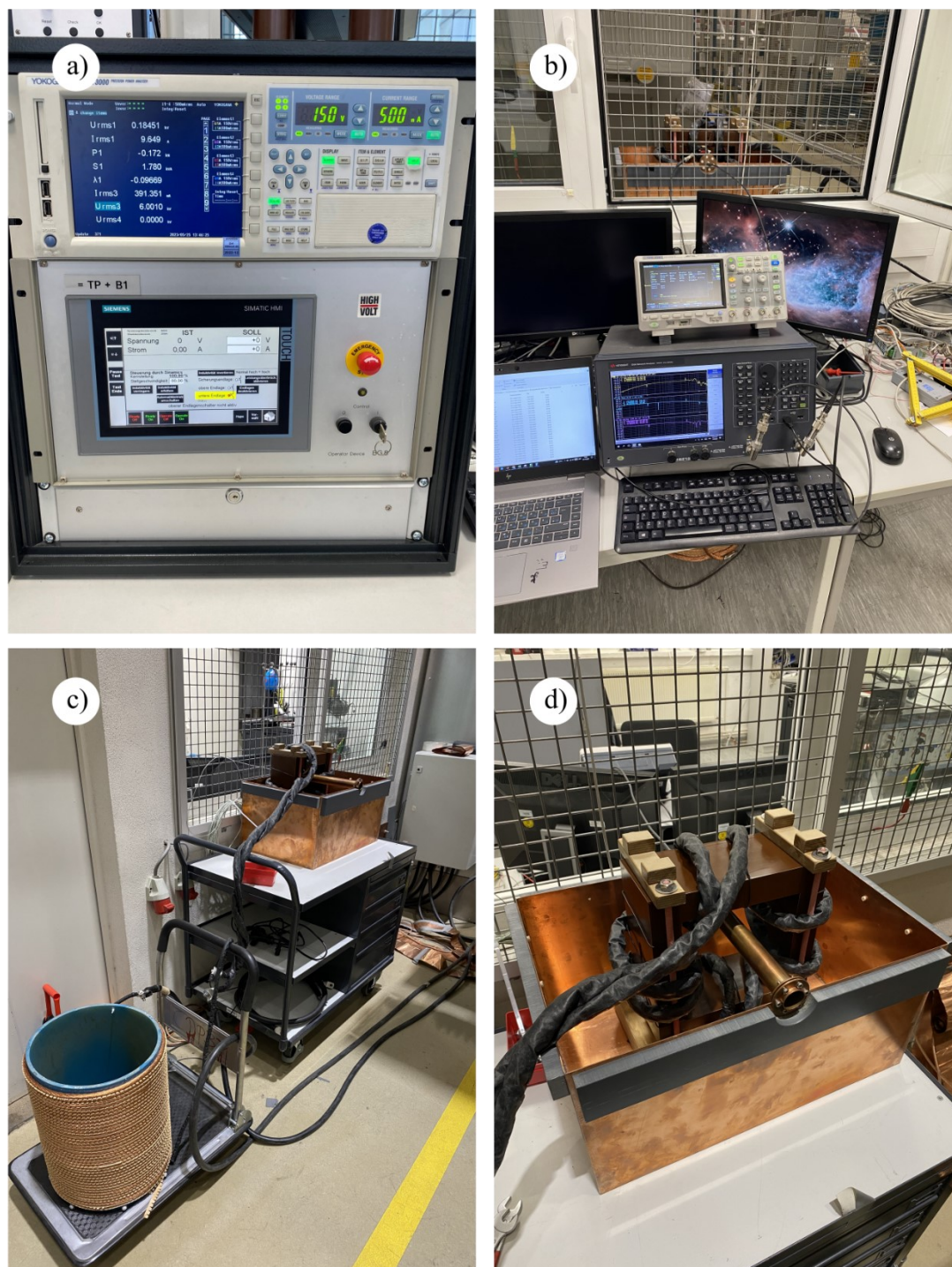
Fig. 4–61 Measurement of HFCT transfer function with superimposed AC power current
