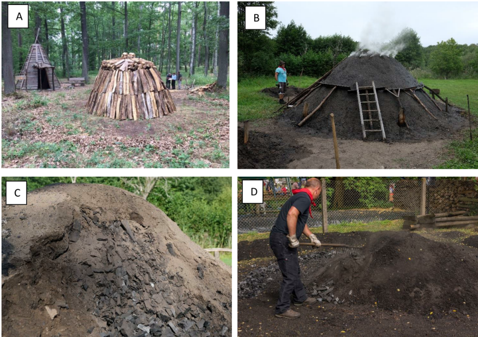
Abbildung 1.1. A – B) Uncovered charcoal hearth wood stack and covered hearth in use (pictures: S. Vane & F. Hirsch). C – D) After the pyrolysis is complete, the hearth is harvested carefully (pictures: A. Bonhage). The pictures have been taken 2018 and 2022 in Brandenburg, Germany and show reconstructions of the historic charcoal hearth operation process.
