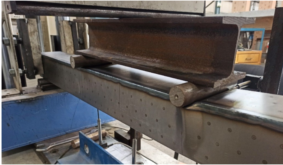
Figure 7.46. Beam 8 back view (flat 1.00 mm + structured 0.5 mm)
