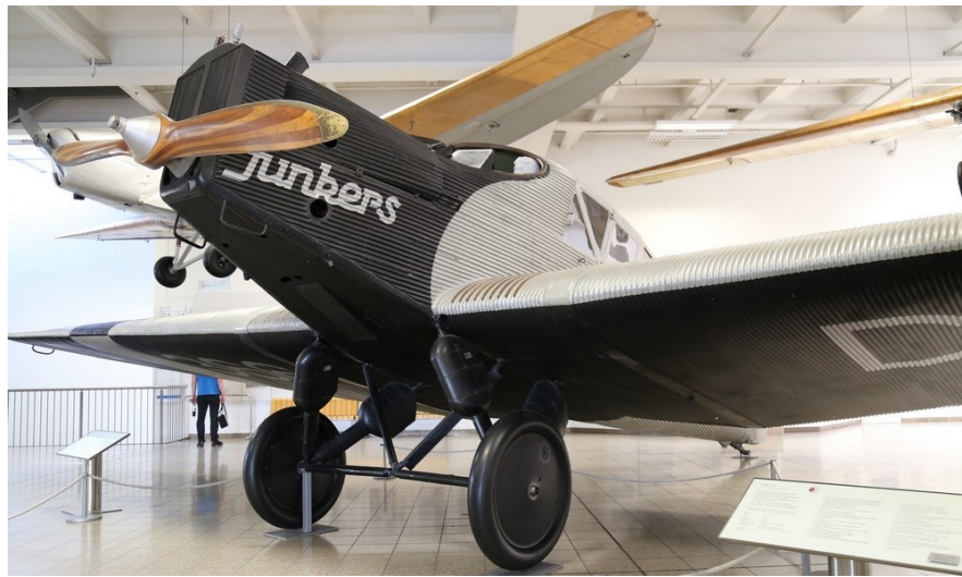
Figure 2.1. Junkers F13 covered with corrugated sheets
