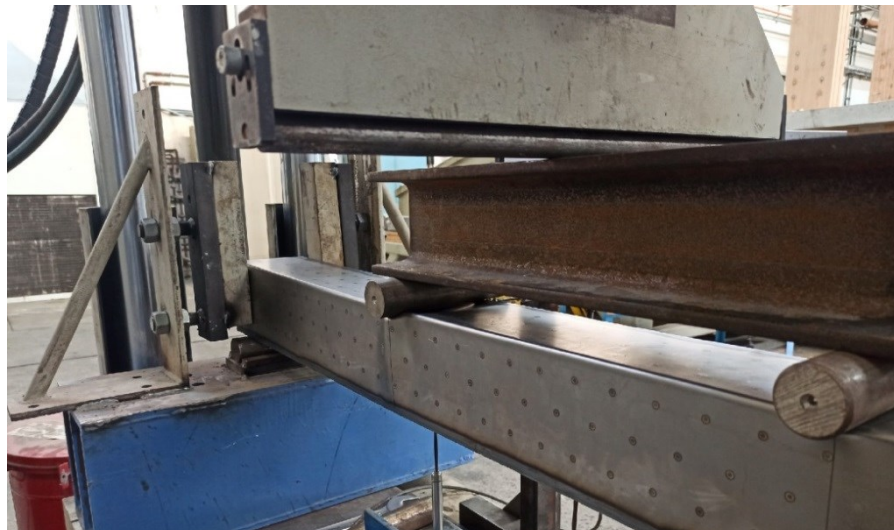
Figure 7.44. Beam 7 back view (flat 1.00 mm + structured 0.5 mm)
