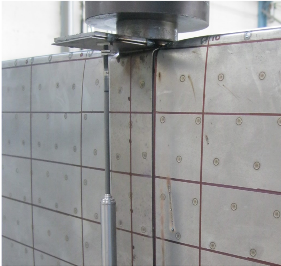
Figure 7.15. Beam 8 back view (flat 1.00 mm + structured 0.50 mm)
