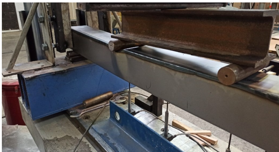
Figure 7.33. Beam 2 back view (flat 1.25 mm)
