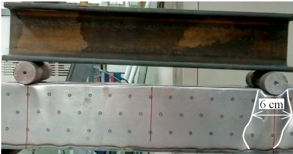
Figure 4.8. Beam 5 buckling area, laboratory experiments
