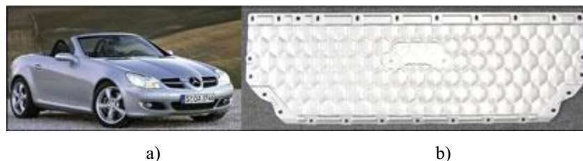
Figure 2.33. Figure Mercedes SLK (a) and vault-structured sheet with a hexagonal staggered pattern (b) [87]
