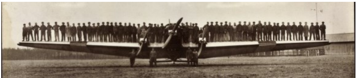
Figure 2.2. Stress-test of a Junkers G-23 plane [26]
