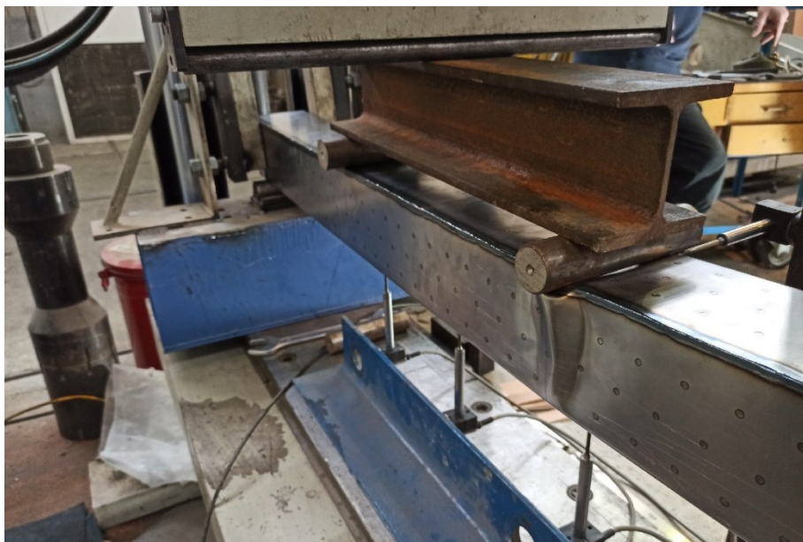
Figure 7.42. Beam 6 back view (flat 0.75 mm + structured 0.5 mm)
