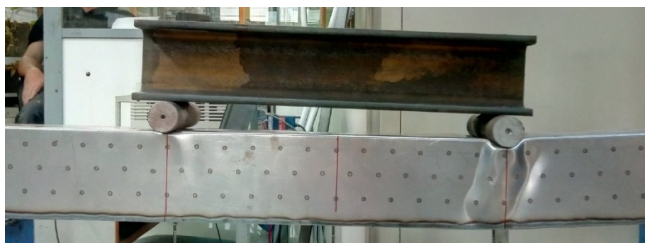
Figure 7.39. Beam 5 front view (flat 0.75 mm + structured 0.5 mm)
