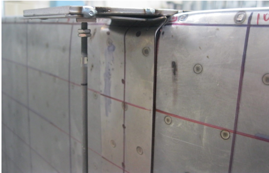
Figure 7.13. Beam 7 back view (flat 1.00 mm + structured 0.50 mm)
