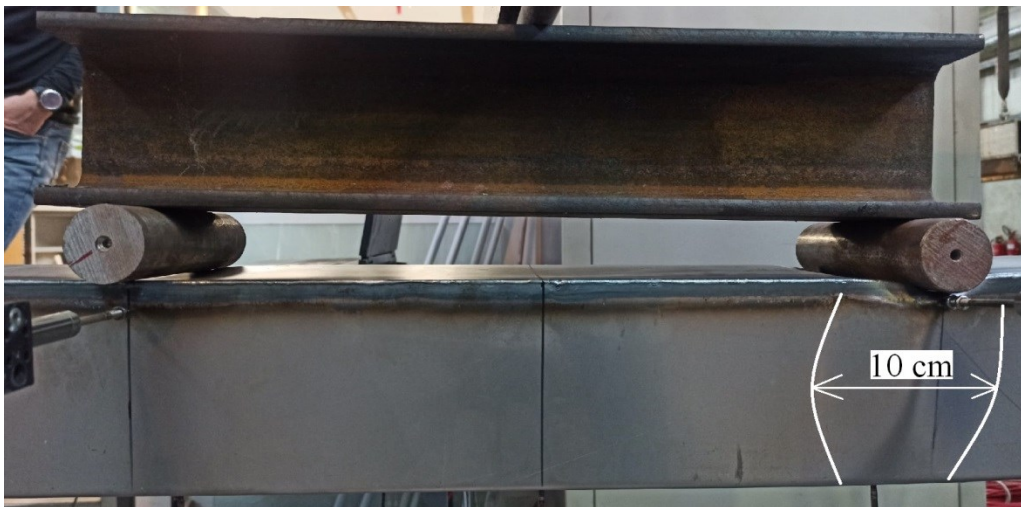
Figure 4.7. Beam 2 buckling area, laboratory experiments
