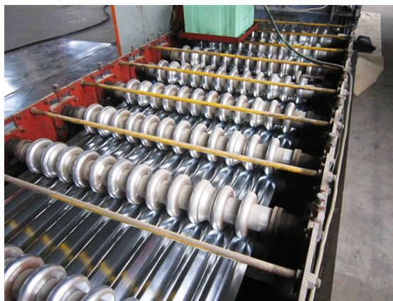
Figure 2.5. Corrugated sheet manufacturing using rotating tools [53]
