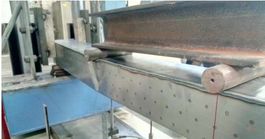
Figure 7.40. Beam 5 back view (flat 0.75 mm + structured 0.5 mm)
