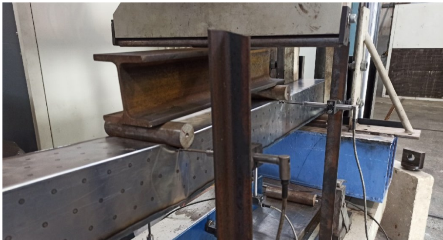
Figure 7.41. Beam 6 side view (flat 0.75 mm + structured 0.5 mm)
