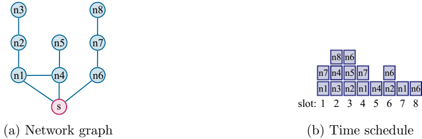
Figure 33: Network graph and time schedule calculated using algorithm by Tsai and Chen.
