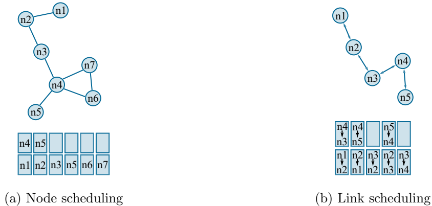
Figure 13: Examples of node and link scheduling.
