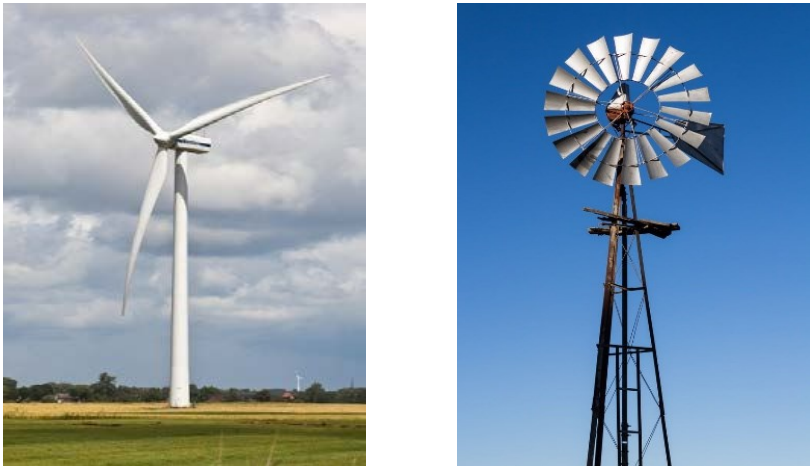
Fig. 1. Horizontal Axis Wind Turbines [3]
