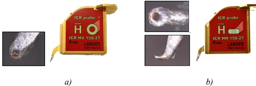
Fig. 11. Langer ICR HV150-27 (a), ICR HH 150-27 (b) EM probes and zoomed-in photos of the probe tips.
