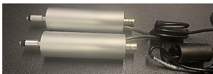
Fig. 8. Riscure EM probes: “high sensitivity” Risc-EMPHS208 (top) and “low sensitivity” Risc-EMPLS211 (bottom).
