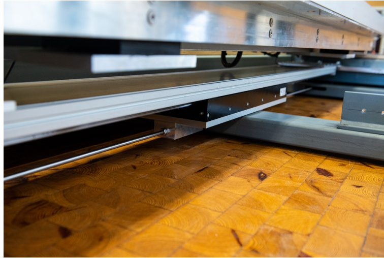
Figure 7.15: Installed NiLAB controlled electric drive of type LM075P (Source: Ralf Schuster, BTU Cottbus-Senftenberg).
