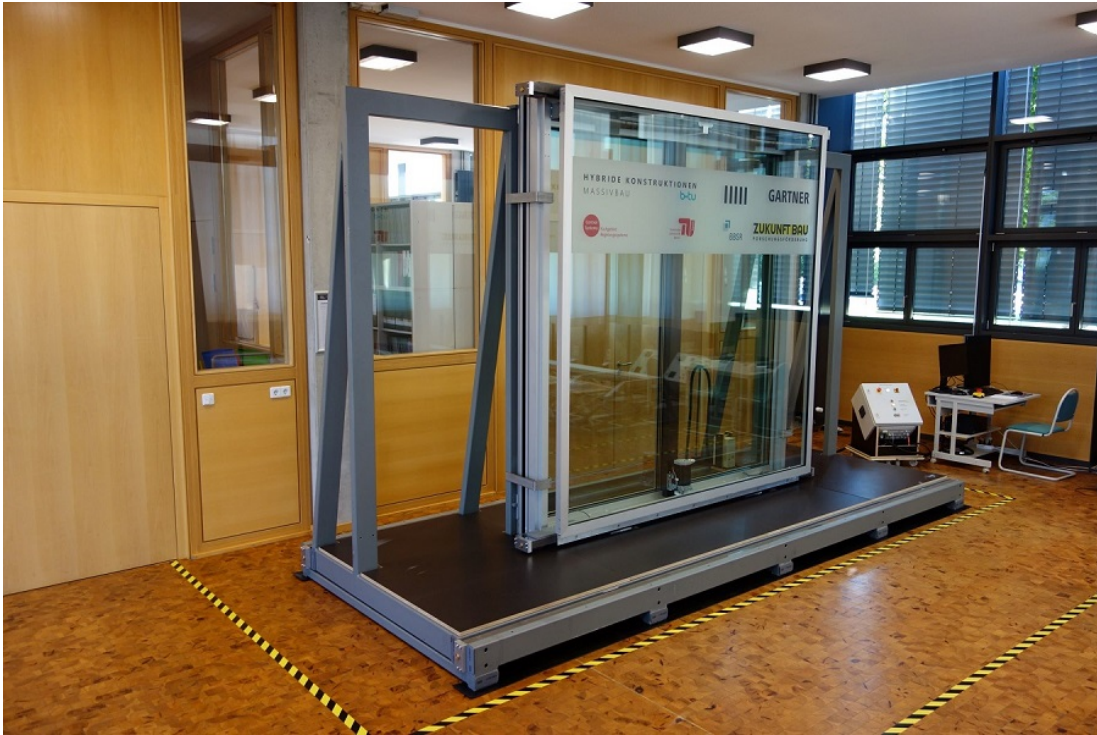
Figure 7.3: Overview of the completed prototype and test rig (Source: Ralf Schuster, BTU Cottbus-Senftenberg).
