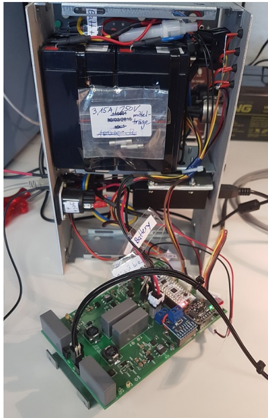
Figure 6.16: Side view of the opened IVE-box (left is the rear view, right is the front view) (Source: Laurenz Wernicke, Technische Universität Berlin).
