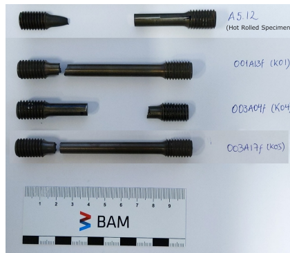
Fig. 4.19: Combined image showing the four studied creep specimens. Photographs of the PBF-LB/M/316L specimen K01 and the hot rolled specimen A5.12 were taken after the XCT scans when the two specimens were already cut for further analysis. Original images provided by Luis Ávila.
