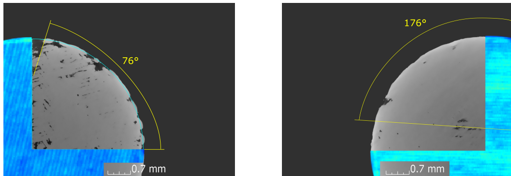
(a) virtual cut taken 60 \mu\text{m} above the bottom of Q8 combined with OT data of layer 200
