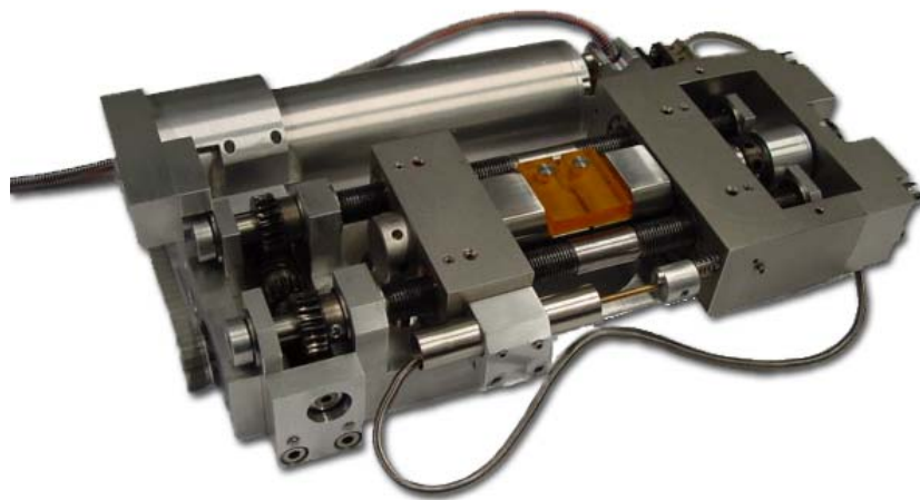
Figure 3.16. Tensile module with CT-specimen.
