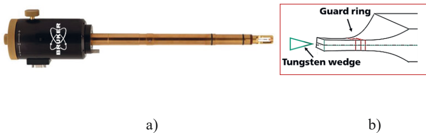
Figure 5.2: (a) Mechanical manipulator (Picoindenter PI95, Bruker Corporation); (b) Scheme of the indentation of the BEoL stack using a tungsten wedge.
