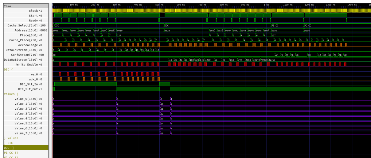
Abb. 56: Timingdiagramm (klein) – MMU - Data-Input Pre-Fetcher
