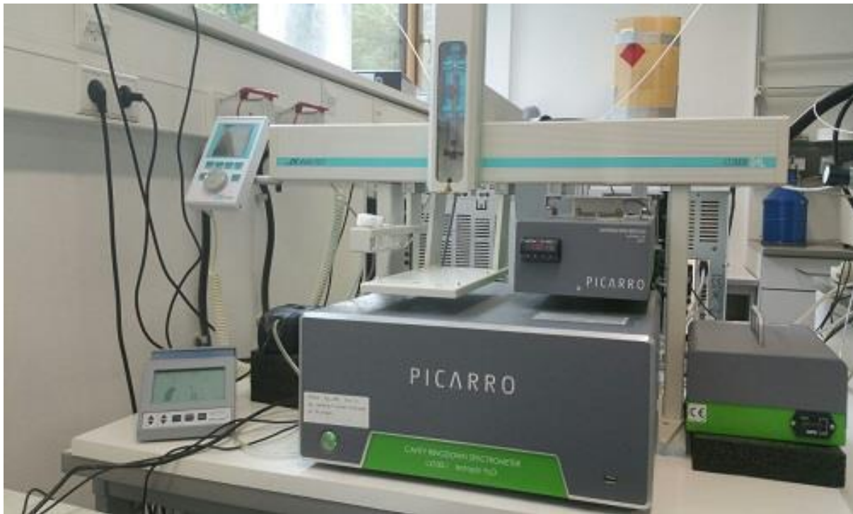
Fig 3.12 laboratory photo of the Picarro L2130-I Cavity Ringdown Spectrometry at the hydrochemistry laboratory of TU Darmstadt.
