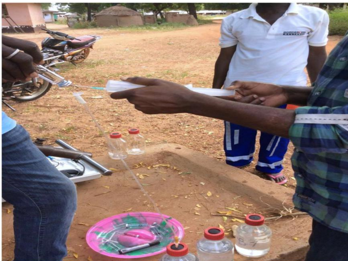
Fig. 3.8 Researcher extracting SF 6 and CFCs gases from the groundwater into 22 mL glass vials (Field Photo 2019)
