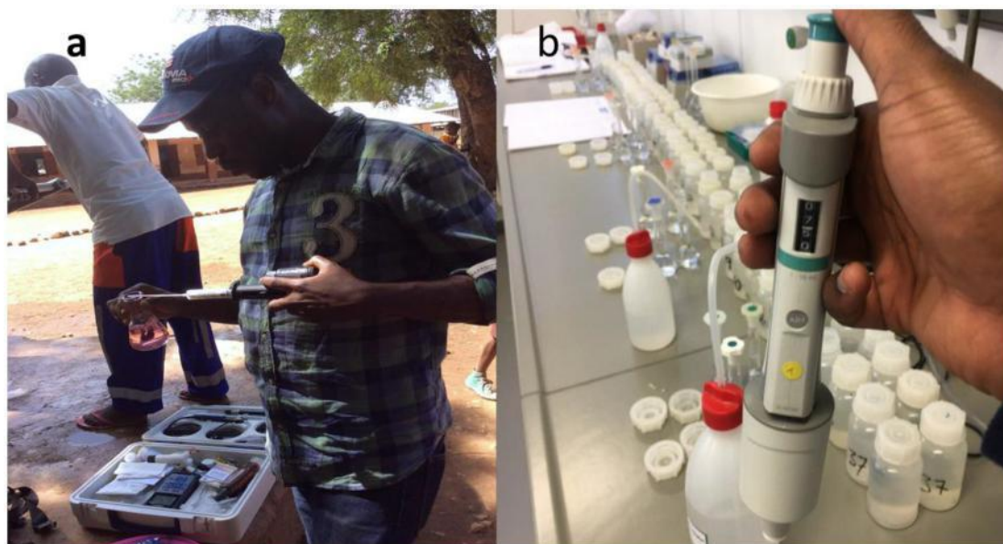
Fig. 3.7 (a) Researcher performing a digital alkalinity titration of groundwater in the field (b) sample preparations of the groundwater samples for hydrochemical analysis
