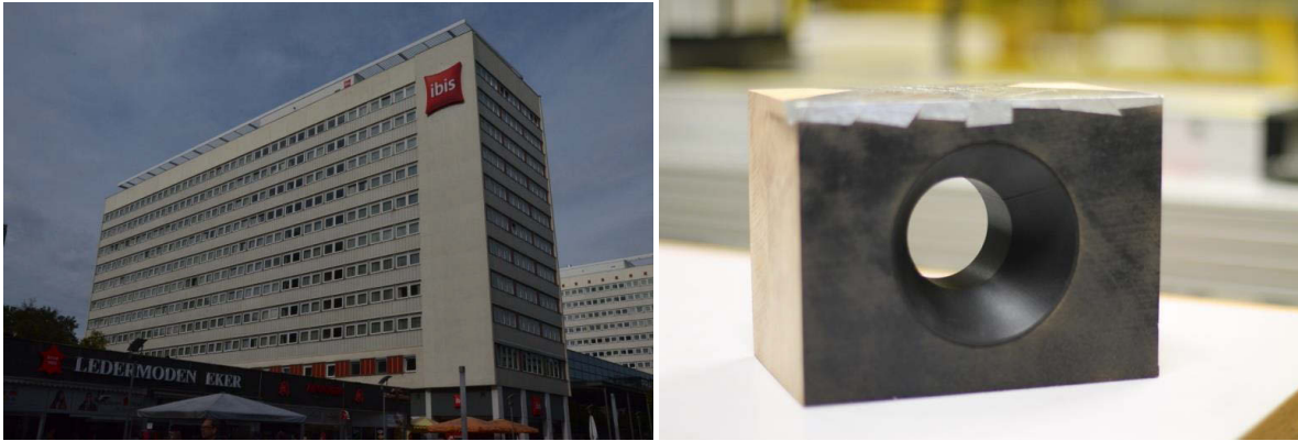
Figure-4.3. Comparison between wind tunnel model and real scale building. Source: own representation.
