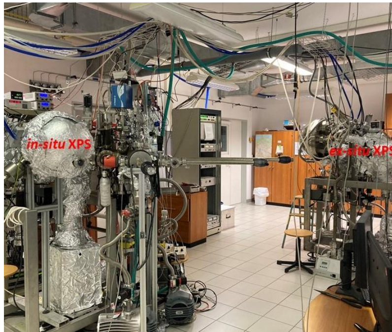
Figure 3.9. In-situ and ex-situ XPS systems in the chair of applied physics and semiconductor spectroscopy of BTU.
