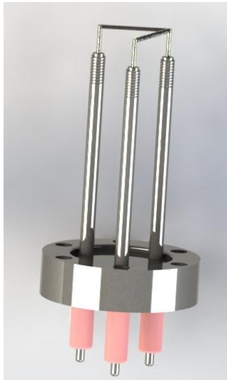
Figure 3.20. Configuration of Ti evaporator system in the BTU's chair of applied physic and semiconductor spectroscopy.
