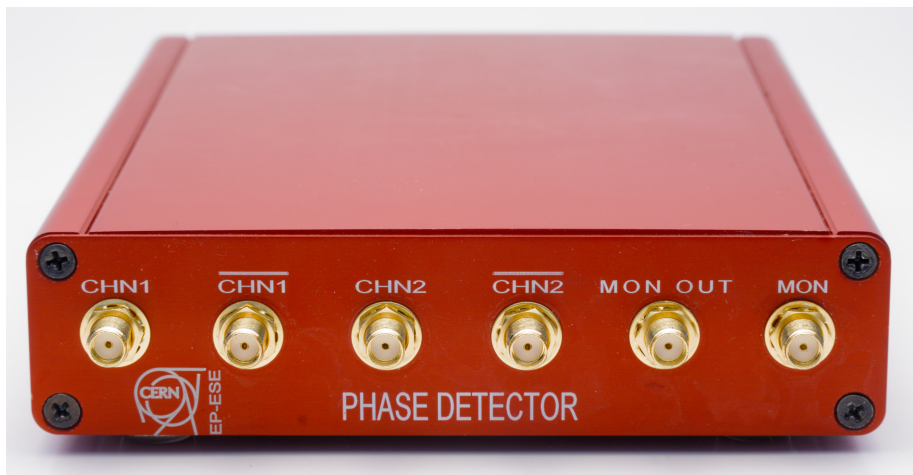
Figure 3.6: Photograph of the manufactured phase measurement system. Differential clock inputs and single-ended voltage outputs are present on the front side of the device, supply voltage is provided from the back.
