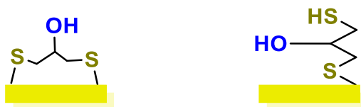
Figure 2.6 Schematic representation of spatial conformation of the two types of binding of DiSH to the gold surface: binding by both thiol groups (left), and binding by only one thiol group (right).
