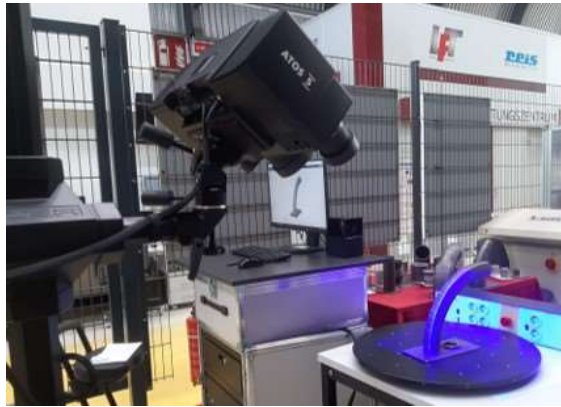
Fig. 17 ATOS 5 system - 3D scanner
