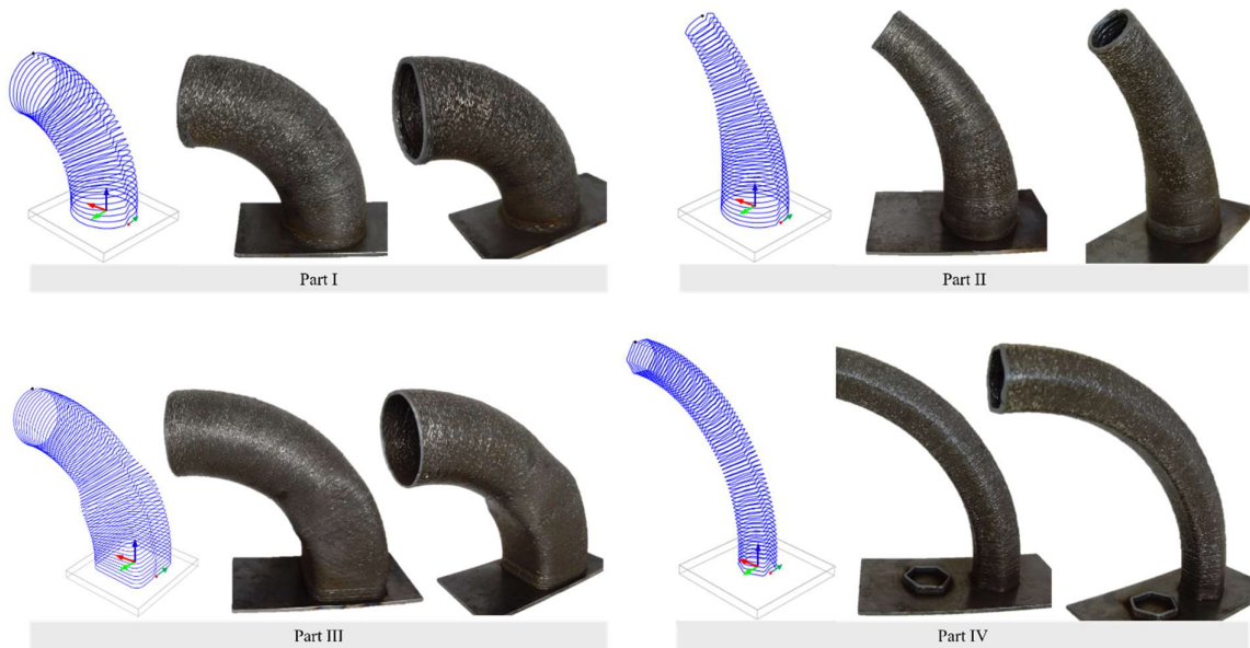
Fig. 78 Tool path and metal part. Only every fifth layer is displayed
