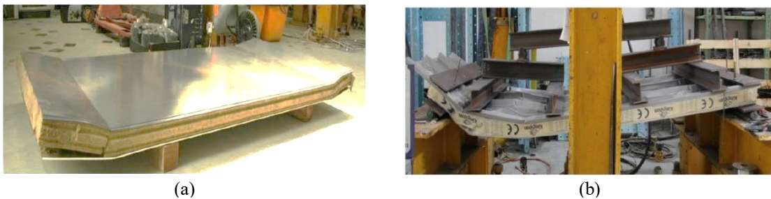
Figure 3.5. Shear failure of a) MW panels and b) PIR panels at normal conditions [8]
