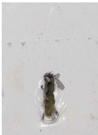
Figure 5.4. Failure of the inner sheet of MW sandwich panels at ambient temperature [8]
