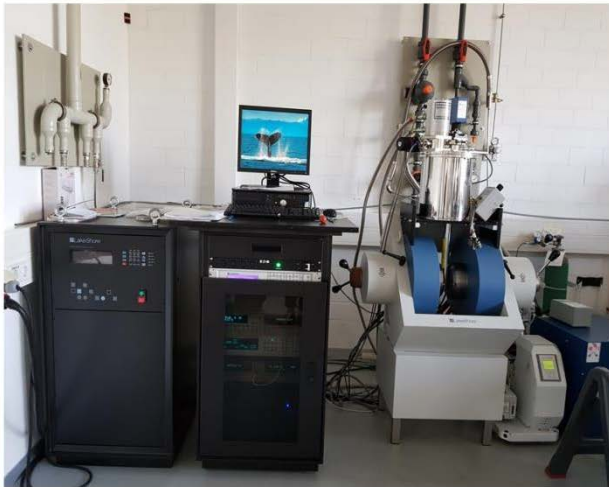
Fig. 3.17. A picture of the Lakeshore 7600 Hall system (left). A schematic illustration of Van der Pauw Hall measurement geometry (right).
