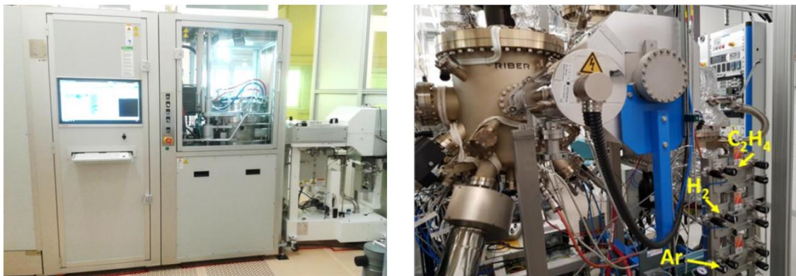
Fig. 3.3. Pictures of the CVD systems that were used for graphene growth in this PhD work.
