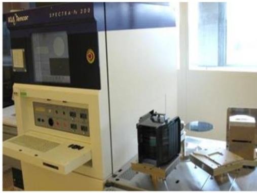
Fig. 3.15. Picture and schematic illustration of the working principle of spectral ellipsometry tool.
