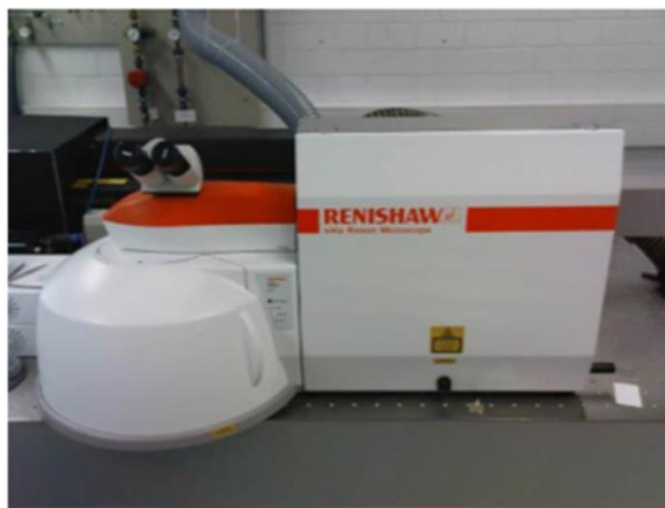
Fig. 3.4. Picture of the Renishaw Raman microscope from the Raman lab at IHP.
