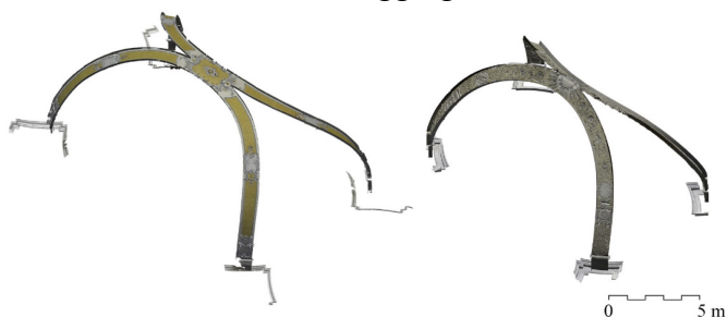
Figure 10. Triangulated scans of the double-curved arches of the church of Vierzehnheiligen (left) and Banz Abbey Church (right); isometric top view.
