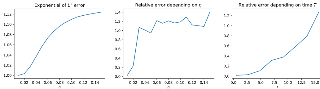
Figure 3.7: Small noise diffusions with vanishing noise coefficient \eta . Left: Exponential of L^2 error between u^* and u^0 depending on \eta for T = 1 . Middle: Relative importance sampling error depending on \eta . Right: Relative importance sampling error depending on T for \eta = 0.005 .
