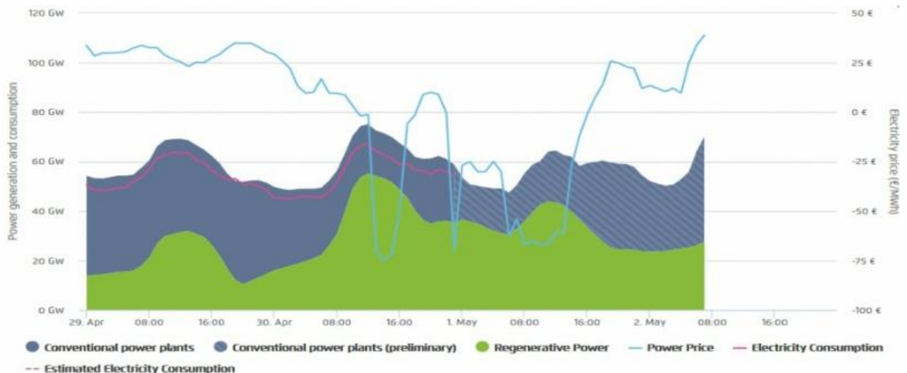
Figure 4. Conventional power generation (gray), renewable (green), electricity demand (pink), and day-ahead electricity prices (blue) [10].
