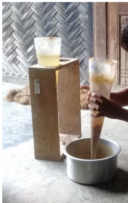
Fig. 10: Taking of sediments from an Imhoff funnel for the determination of the dry mass of suspended sediments (photo: Nils Kreber)
