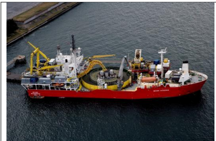
Fig.12: Special Ship for the laying of undersea cables [13]
