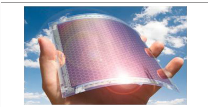
Figure 2. Flexible dye-sensitized solar cell [10]
