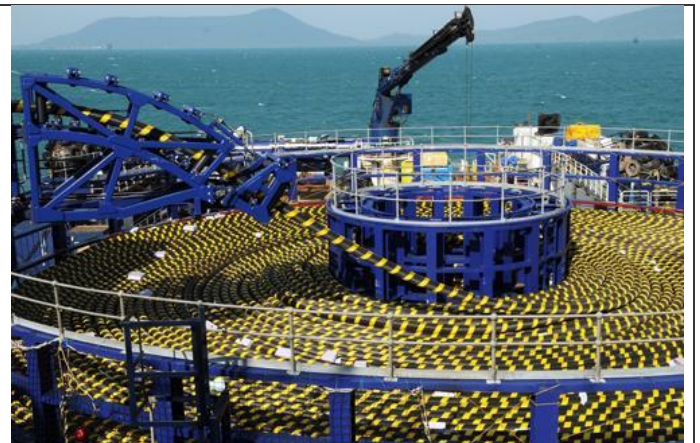
Fig. 13: Deck of the ship with the undersea cable [14]
