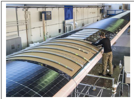
Fig. 1. Construcion of wing
