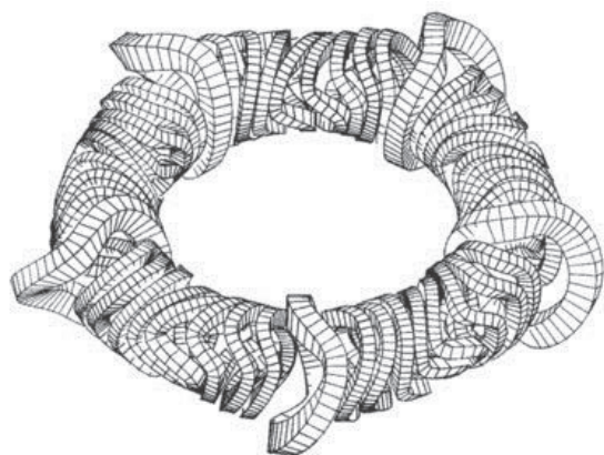
Fig.2: Magnets and plasma of Wendelstein 7-AS stellarator
