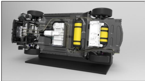
Figure 5: FCV’s propulsion system [7]
