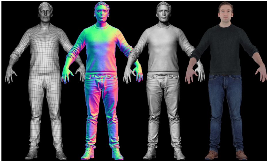
Figure 4.1: Sample 3D-scan of a male human body, f.l.t.r 3D-mesh, displacement map, 3D mesh with applied displacement maps, render with material properties and texture applied [Ten19].
