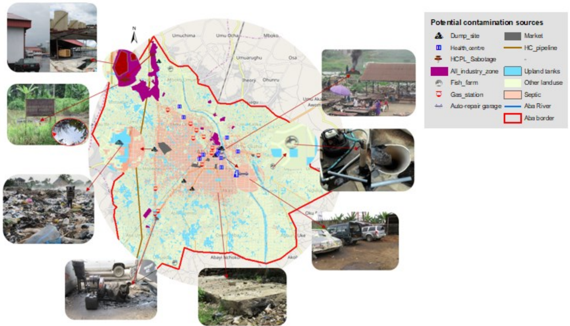
Fig 5-9: Map of land use hotspot showing potential contamination sources overlaid on the urban built-up class and its interaction with some of the upland depression derived from the topographic index map.
