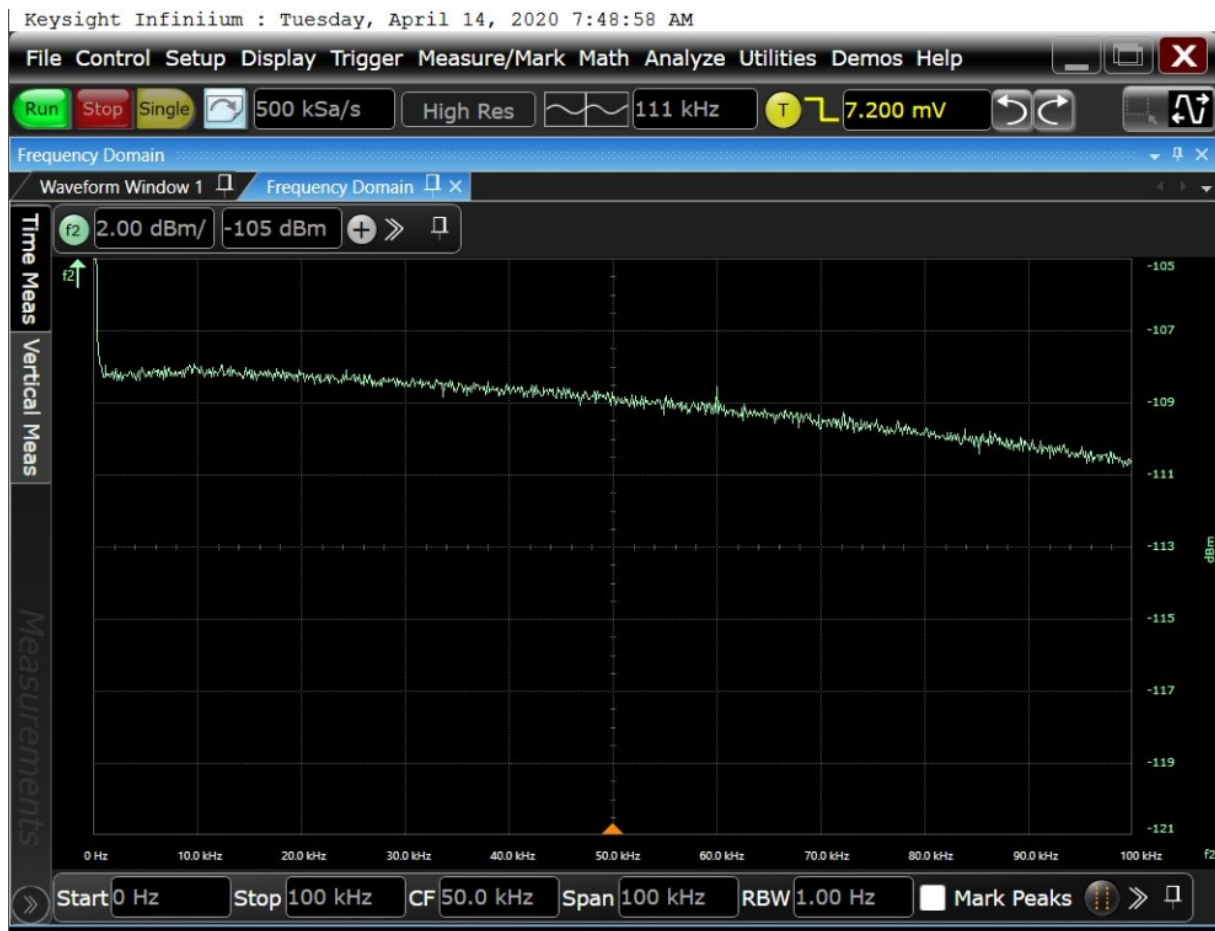
Figure 231- Keysight Scope / LNA Instrument Noise Floor (FFT)
