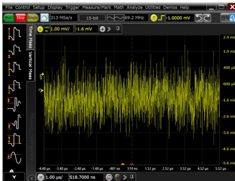
Figure 250 - Breakdown Voltage Waveforms at 2mA Breakdown Current (2N2222A)
