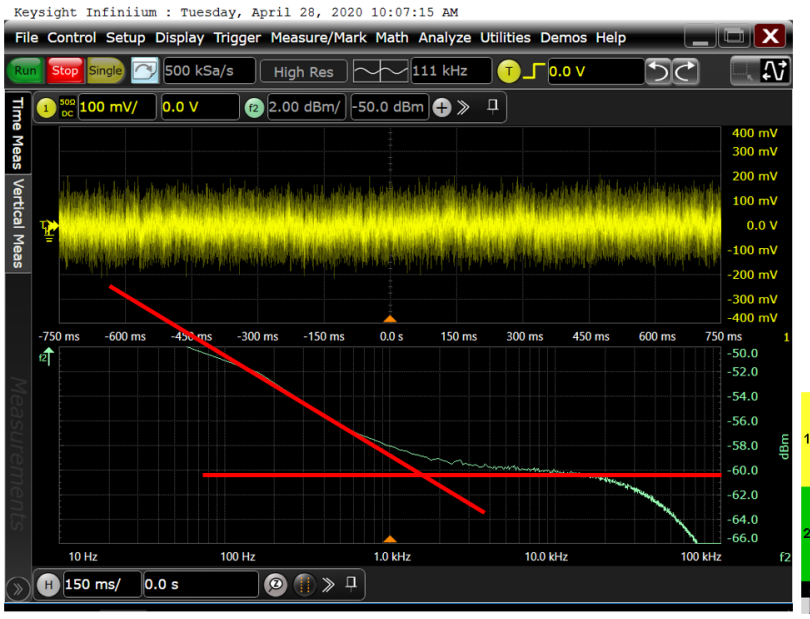
Figure 240 - Noise of an 2N2222A Transistor in Deep Saturation at 5mA I_C
