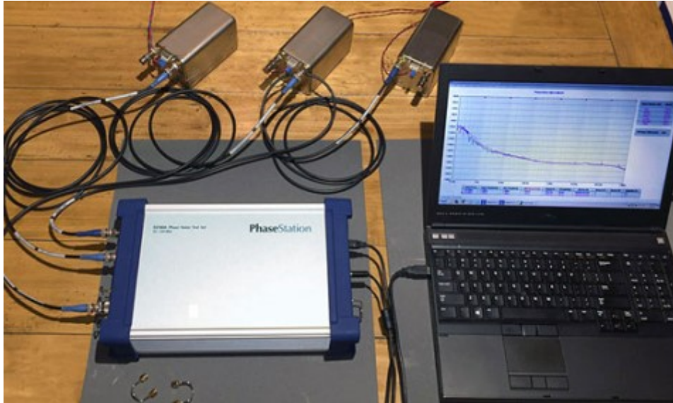
Figure 122 - Test Setup for a 3-Oscillator Correlation Phase Noise Measurement Picture from [12]
