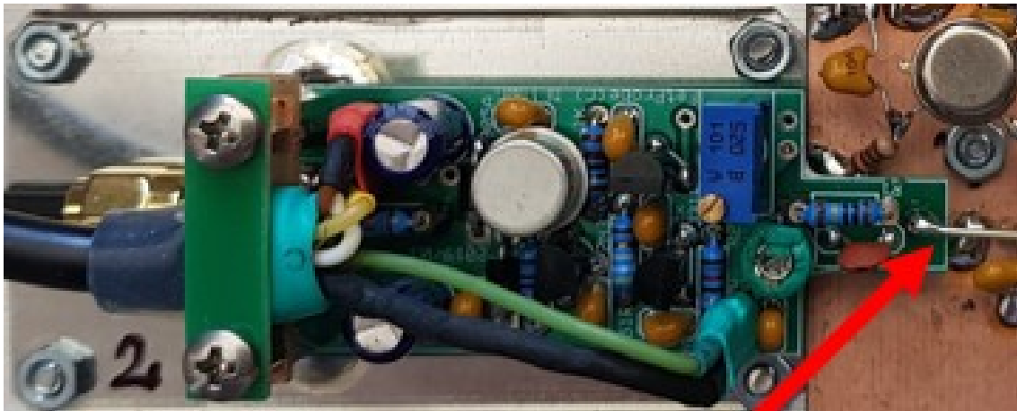
Figure 103 - Photo of a FET Probe in a Test Oscillator
