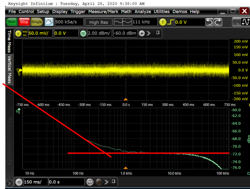
Figure 238 - Noise of an 2N2222A Transistor in Deep Saturation at 500uA I_C
