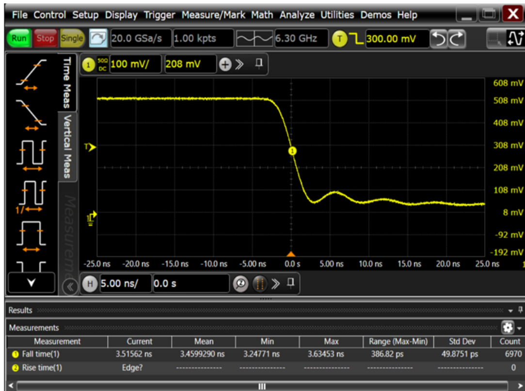
Figure 106 - Fall Time of the FET Probes
