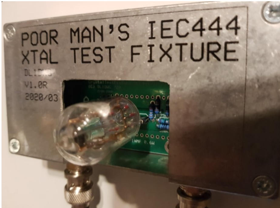
Figure 204 – Self-made Low HF IEC444 Crystal Test Fixture
