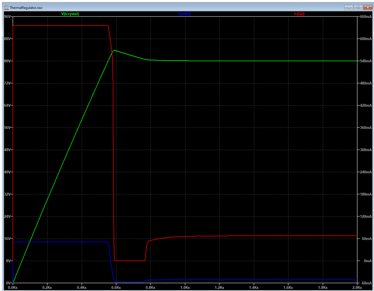
Figure 144 - Heater Current and Crystal Sense Voltage over Time. The red curve is the collector current of the heater transistor, the green curve is the crystal temperature, and the blue curve is the op amp output voltage.
