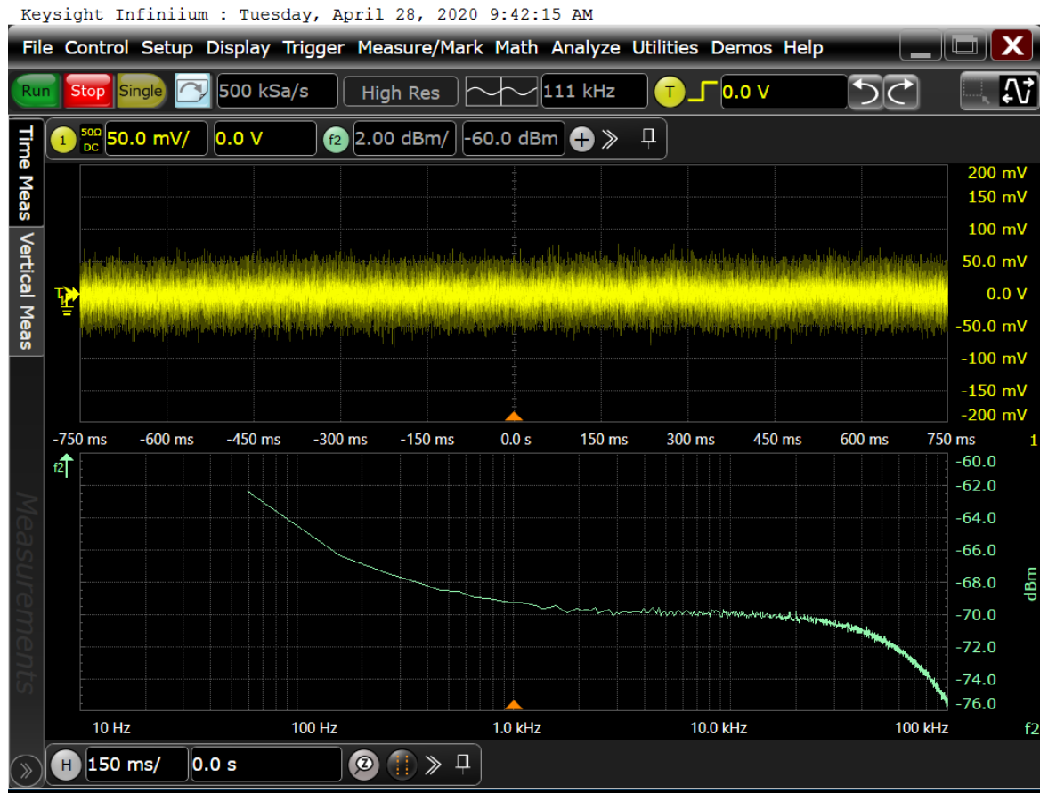
Figure 235 - 2N2222A Noise Floor (500 \mu A/4V)
