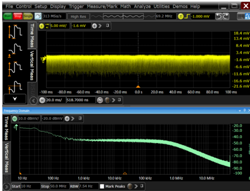
Figure 251 - Breakdown Noise Spectrum at 200nA (2N2222A)
