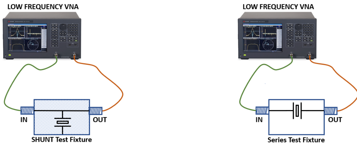
Figure 197 - Crystal Parameter Measurements Using a VNA Photos of Instruments from Keysight Website
