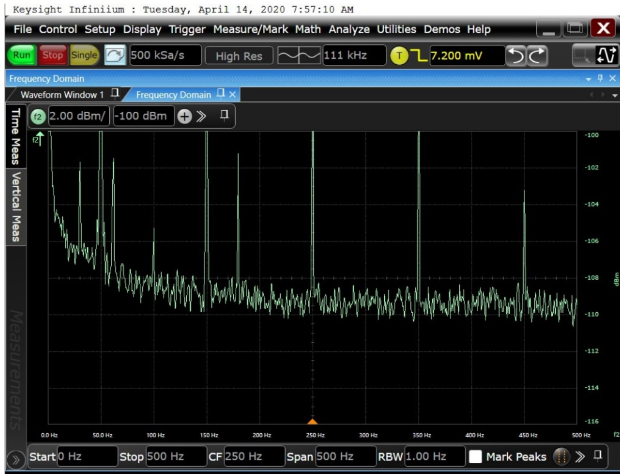
Figure 232 - Keysight Scope / LNA Instrument Noise Floor (FFT) Zoom to LF
