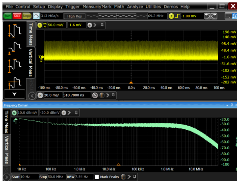
Figure 252 - Breakdown Noise Spectrum at 20uA (2N2222A)
