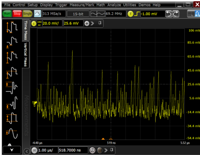
Figure 249 - Breakdown Voltage Waveforms at 20uA Breakdown Current (2N2222A)
