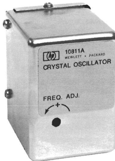
Figure 185 - The Packaged HP10811A Crystal Oscillator Picture from HP Journal [1]
