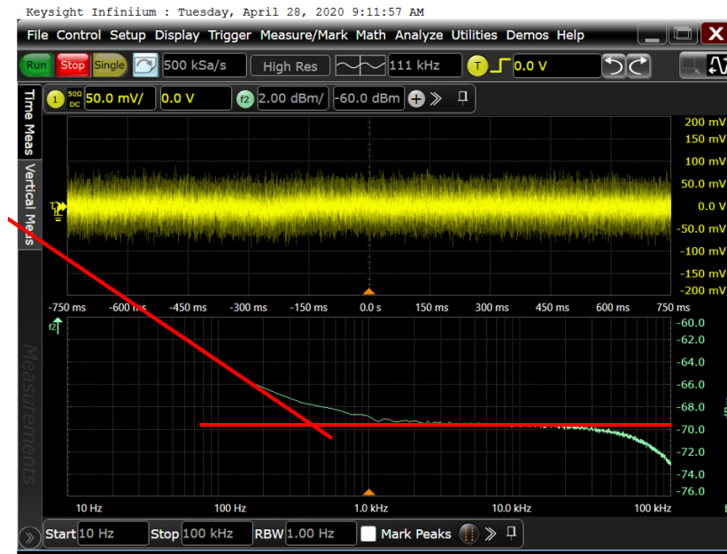
Figure 237 - Noise of an 2N2222A with no Saturation at 500uA I_C
