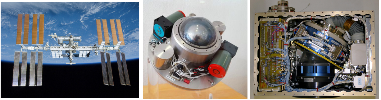
Figure 3: (left) International Space Station (ISS) (source: ESA), (middle) GeoFlow core facility (source: LAS/BTU), (right) GeoFlow container (source: LAS/BTU).
