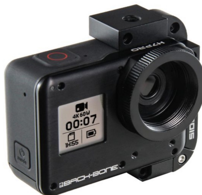
Figure 4.3: Back-bone modified GoPro Hero 7 Black. Source: www.back-bone.ca .
