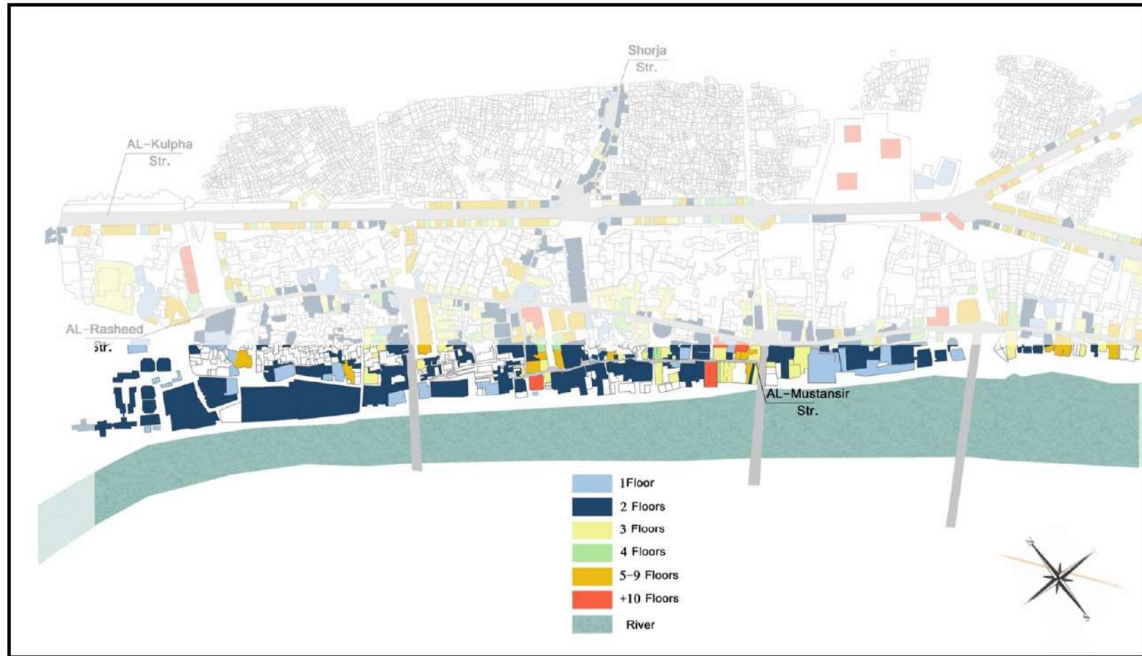
Fig. (5.14): - The height survey for the buildings along Sarai street & AL-Mustansir street in the old city of Baghdad, Source: Drawn by the Author based on personal survey accompanied with reviewing and editing a survey that was done in 2008 for both AL-Rasheed street and AL-Mustansir street cited in Abdul Hadi.T 2017,14, See Fig. (47) in Appendix I in A3 Size.
