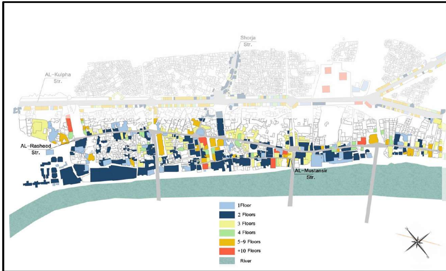
Fig. (5.22): - The Height survey for the buildings along AL-Rasheed street in the old city of Baghdad, Source, drawn by the Author based on personal survey accompanied with reviewing and editing a survey that was done in 2008 for both AL-Rasheed street and AL-Mustansir street cited in Abdul Hadi.T 2017,14, See Fig. (48) in Appendix I in A3 Size.
