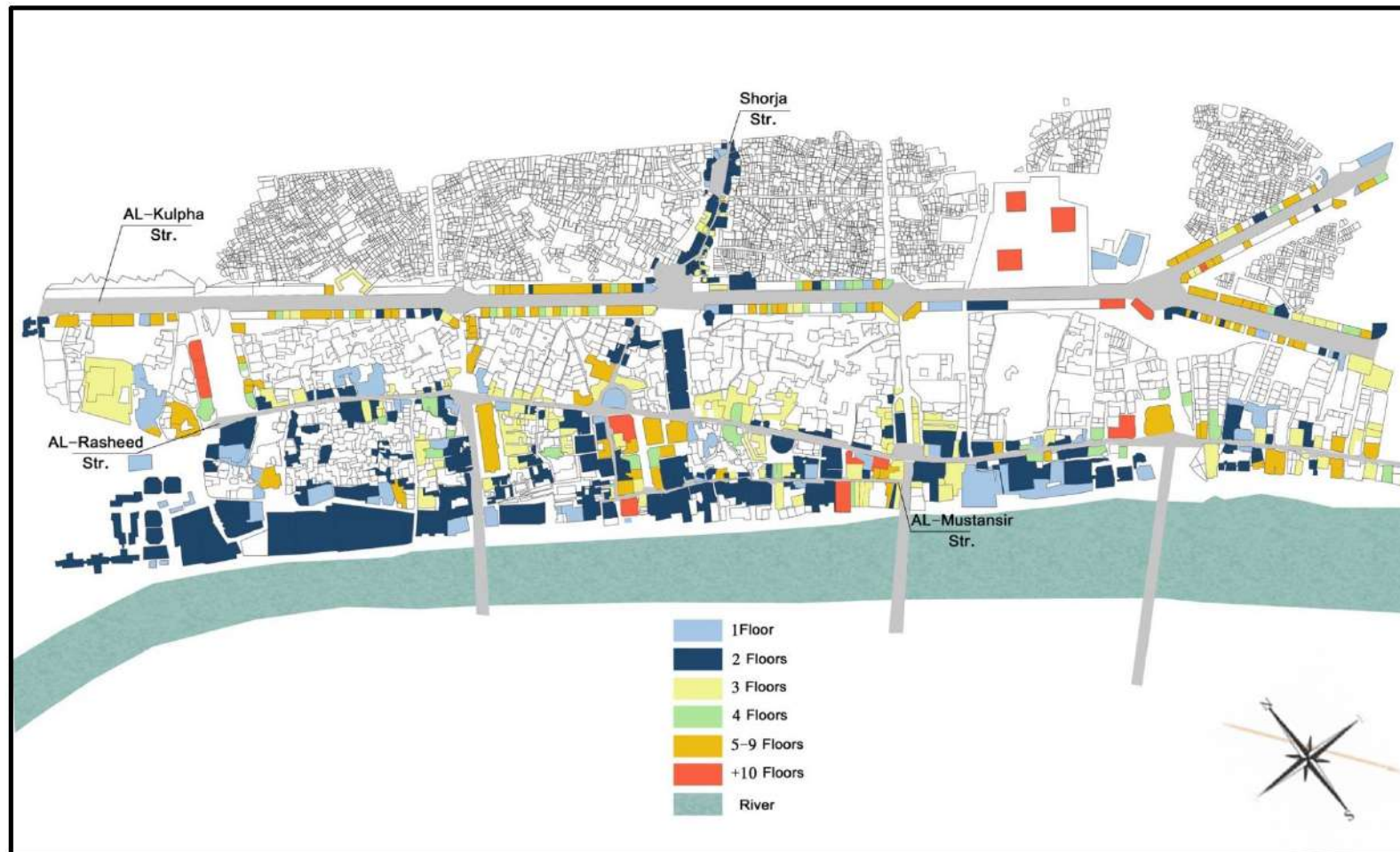
Fig. (5.8): - The height survey for the buildings along the main pedestrian streets (Shorja and AL-Mustansir streets) and car streets (AL-Rasheed street & AL-Khulapha street) in the old city of Baghdad, Source: Drawn by the Author based on personal survey accompanied with reviewing and editing a survey that was done in 2008 for both AL-Rasheed street and AL-Mustansir street cited in Abdul Hadi.T 2017,14, See Fig. (45) in Appendix I in A3 Size.
