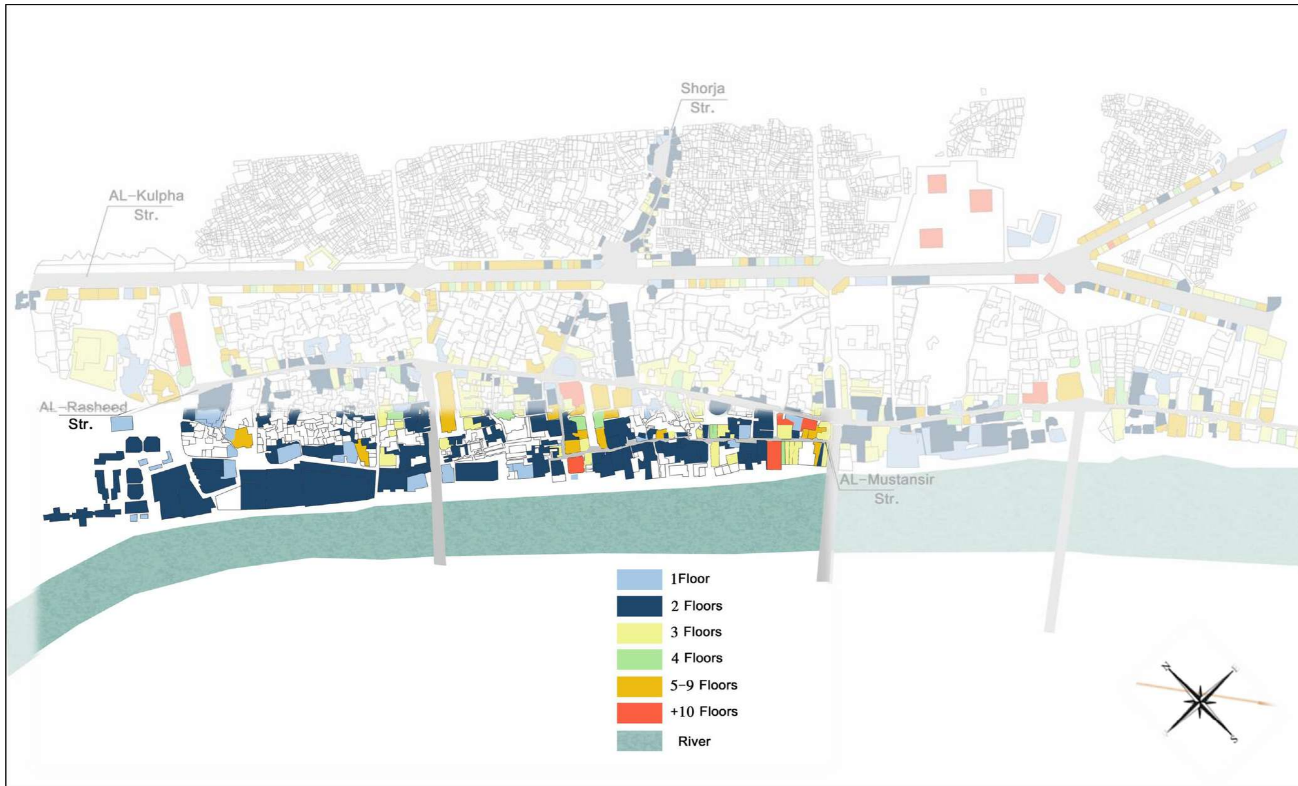
Figure -47-: The height survey for the buildings along Sarai street & AL-Mustansir street in the old city of Baghdad, Source: Drawn by the Author based on personal survey accompanied with reviewing and editing a survey that was done in 2008 for both AL-Rasheed street and AL-Mustansir street cited in Abdul Hadi.T 2017:14.
