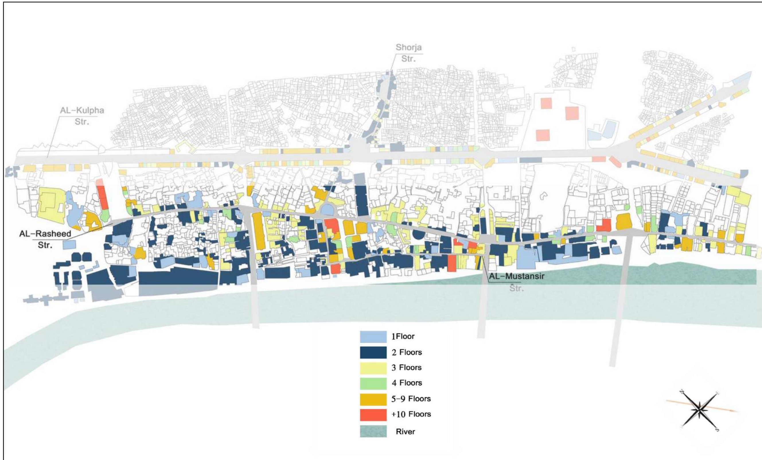
Figure -48-: The height survey for the buildings along AL-Rasheed street in the old city of Baghdad, Source: Drawn by the Author based on personal survey accompanied with reviewing and editing a survey that was done in 2008 for both AL-Rasheed street and AL-Mustansir street cited in Abdul Hadi.T 2017:14.
